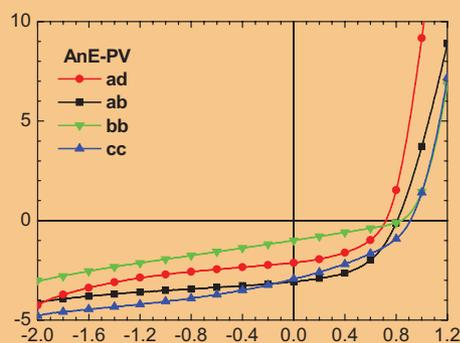
IV-characteristics of partly optimized photovoltaic devices based on [6,6]-phenyl C<sub>61</sub> butyric acid methyl ester (PCBM) blends with a blending ratio of 1:1 under solar simulator illumination.
