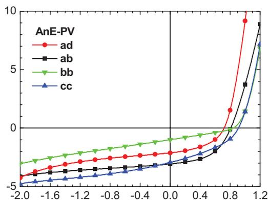
**Figure 2** (online colour at: [www.pss-a.com](http://www.pss-a.com)) IV-characteristics of partly optimized photovoltaic devices based on polymer:PCBM blends with a blending ratio of 1:1 under solar simulator illumination.
