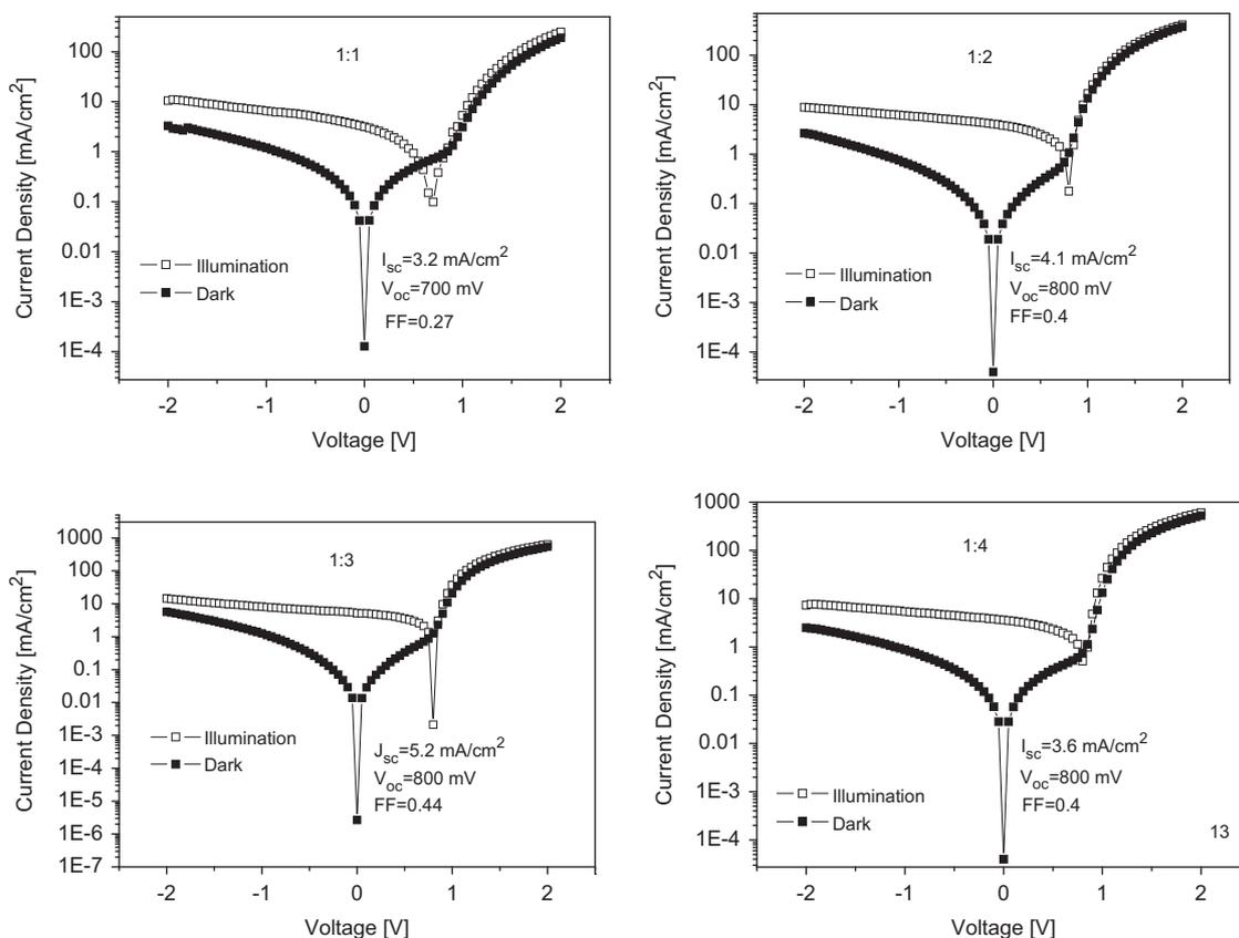
Fig. 7. Current–voltage characteristics of **P2**:PCBM 1:1, 1:2, 1:3 and 1:4 ratios.
