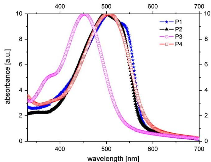
Fig. 2. Optical absorption spectra of thin films of pristine polymers **P1**–**P4**.
