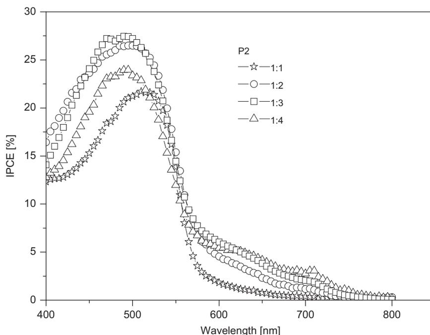
Fig. 9. IPCE for **P2**:PCBM blend solar cells with different wt ratios..
