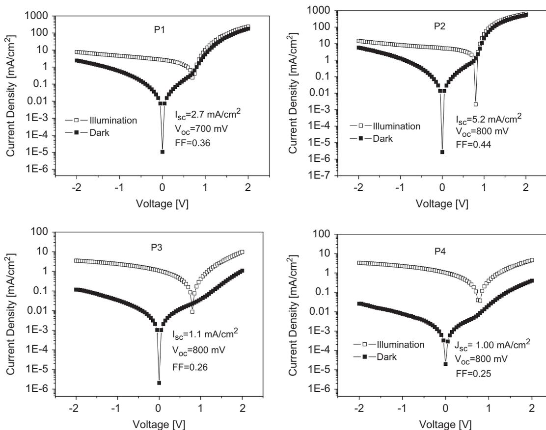
Fig. 3. Current–voltage characteristics of **P1**:PCBM, **P2**:PCBM, **P3**:PCBM and **P4**:PCBM with 1:3 wt ratio.
