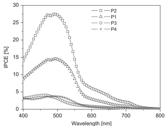
**Fig. 5.** IPCE spectra of the solar cells (**P1**:PCBM, **P2**:PCBM, **P3**:PCBM, **P4**:PCBM blends with 1:3 ratio).
