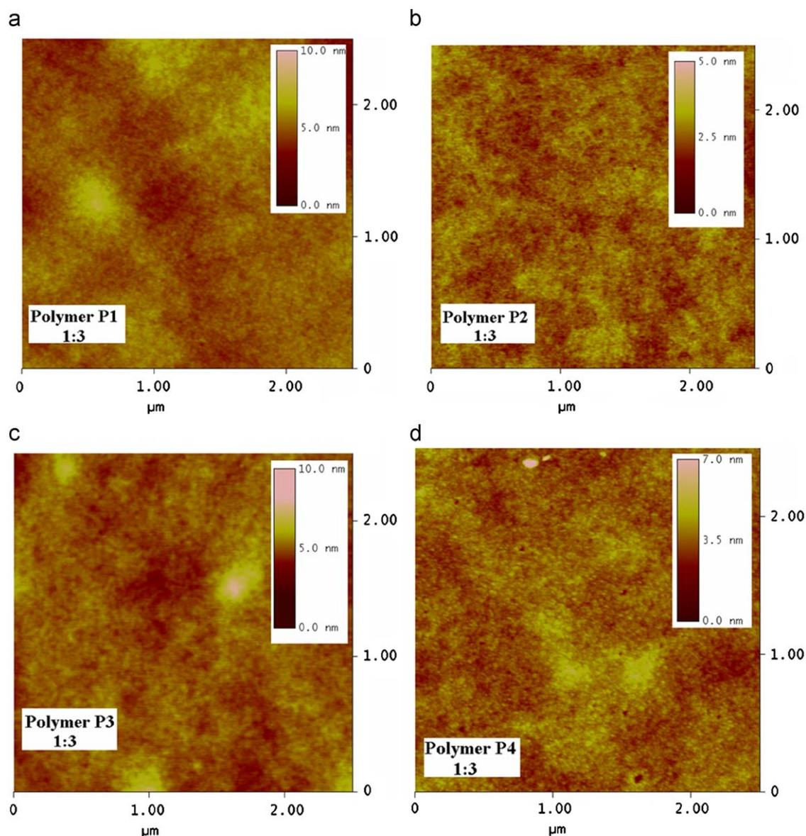
**Fig. 4.** AFM images of blend films of different polymers with PCBM spin cast from chlorobenzene (a) polymer **P1**:PCBM, (b) polymer **P2**:PCBM, (c) polymer **P3**:PCBM and (d) polymer **P4**:PCBM with 1:3 wt ratio.
