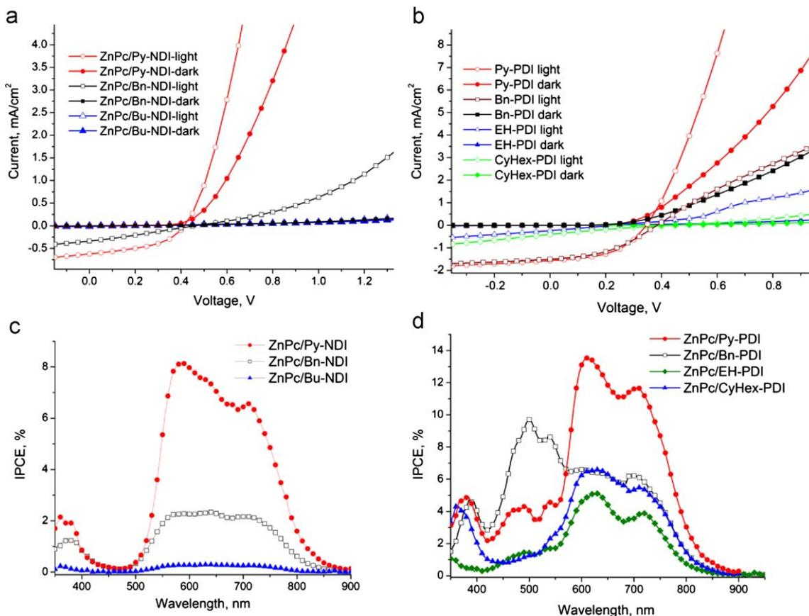
Fig. 5.  $I$ - $V$  curves (a, b) and IPCE spectra (c, d) for bilayer cells comprising ZnPc/NDI (a, c) and ZnPc/PDI (b, d) material combinations.
