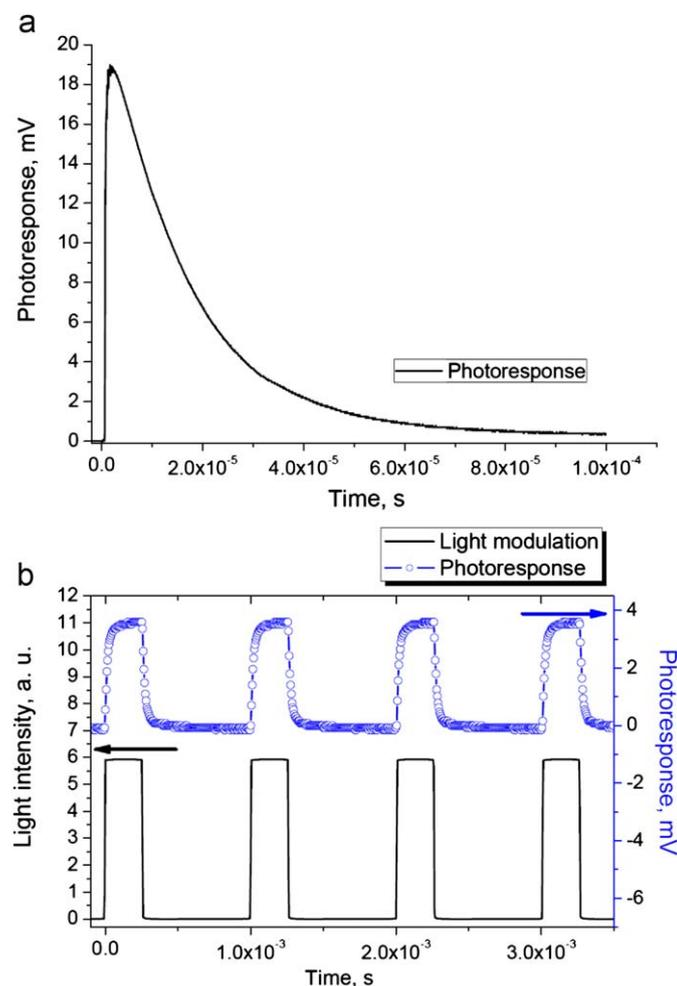
**Fig. 6.** The photoresponse of a ZnPc/Py-PDI bilayer cell induced by single 10 ns light pulse from a 337 nm nitrogen laser (a). Detection of the light from a 460 nm light emitting diode modulated with a 4 KHz frequency by the ZnPc/Py-PDI device (b).
