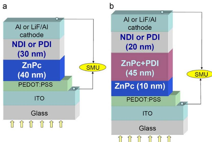
Fig. 4. Schematic layouts of simple bilayer (a) and diffusion bilayer (b) photovoltaic devices.
