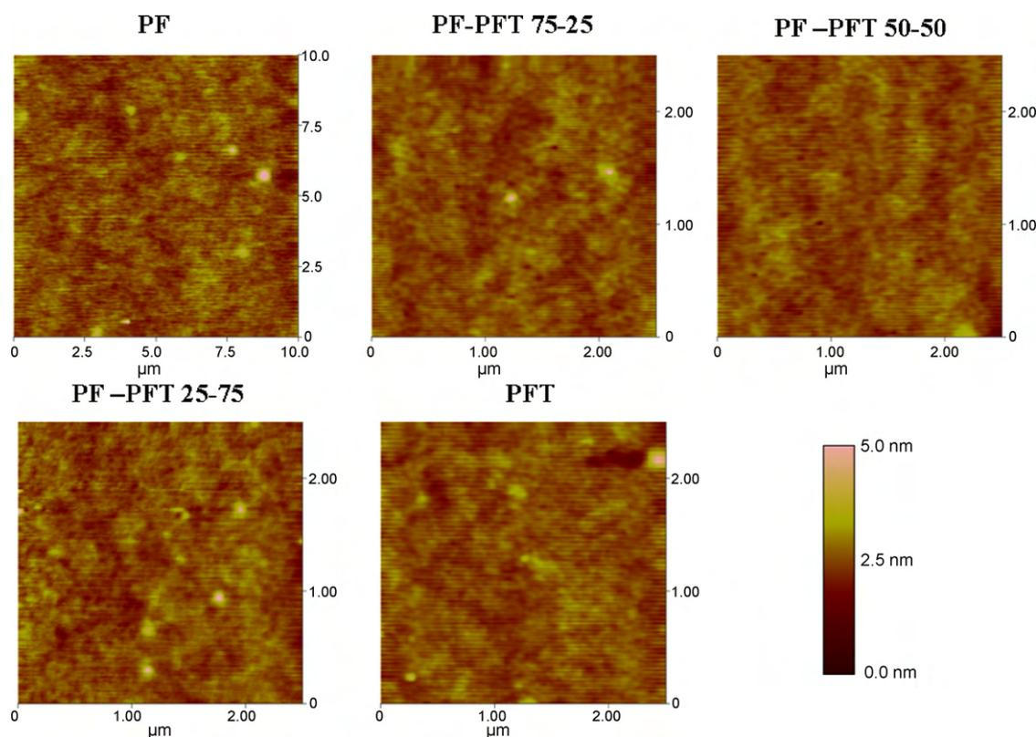
**Fig. 6.** Tapping mode AFM of films of different polymers mixed with 80 wt% of PCBM. The scanning area is  $2.5 \mu\text{m} \times 2.5 \mu\text{m}$ .
