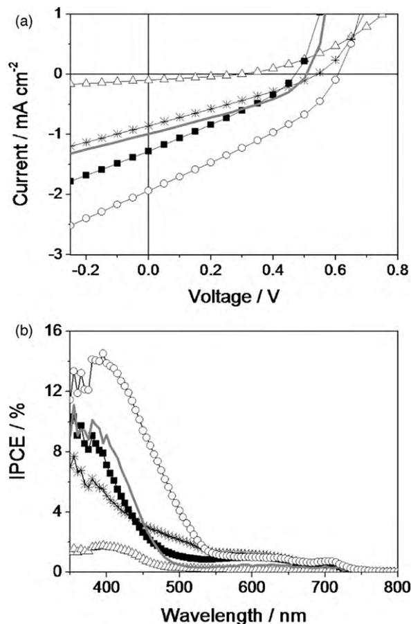
**Fig. 7.**  $J$ - $V$  curves under 100 mW cm<sup>-2</sup> (a) and IPCE characteristics (b) for devices assembled with 80 wt% of PCBM, ~0.1 cm<sup>2</sup> active area, annealed at 130 °C for 5 min: (Δ) PF, (■) PF-PFT 75-25, (●) PF-PFT 50-50, (○) PF-PFT 25-75 and (\*) PFT.
