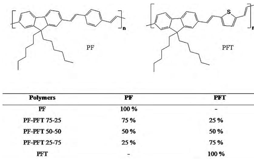
Fig. 1. Structure of the polymers investigated in this work.
