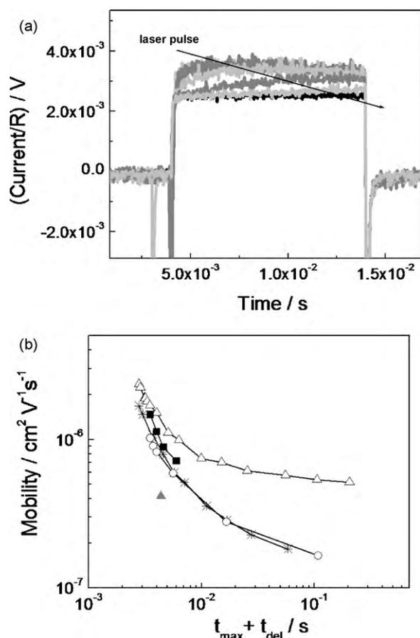
**Fig. 5.** Photo-CELIV current transients recorded for various delay times  $t_{\text{del}}$  between the laser pulse and the triangle-shaped voltage pulse (a) and charge carrier mobility calculated for the different polymers: ( $\Delta$ ) PF, ( $\blacksquare$ ) PF-PFT 75–25, ( $\blacktriangle$ ) PF-PFT 50–50, ( $\circ$ ) PF-PFT 25–75 and ( $*$ ) PFT.
