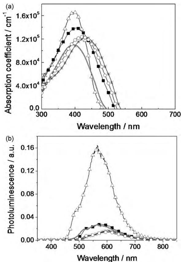
Fig. 3. Absorption coefficient (a) and photoluminescence (b) spectra obtained for polymer films of ~70–90 nm, deposited onto ITO-glass: (Δ) PF, (■) PF-PFT 75–25, (▬) PF-PFT 50–50, (○) PF-PFT 25–75 and (\*) PFT.
