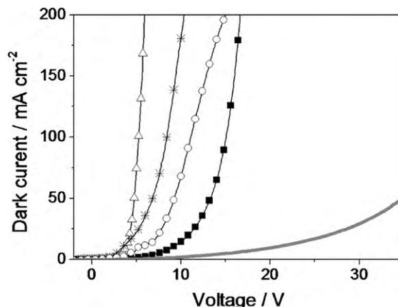
**Fig. 4.**  $J$ – $V$  characteristics in the dark for devices with the following configuration: ITO | PEDOT:PSS | polymer | LiF | Al, where the polymer film thickness is about ~80–100 nm and the active area is ~0.1 cm<sup>2</sup>. ( $\Delta$ ) PF, ( $\blacksquare$ ) PF-PFT 75–25, ( $\bigcirc$ ) PF-PFT 50–50, ( $\ast$ ) PF-PFT 25–75 and (—) PFT.
