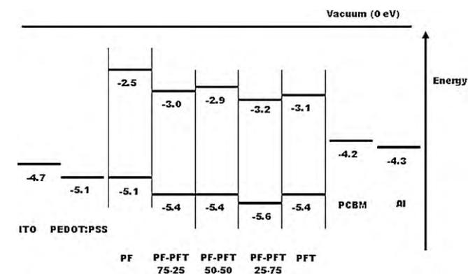
Fig. 2. Energy level diagram showing HOMO and LUMO levels for the polymers, LUMO of PCBM and the work function of the electrodes.
