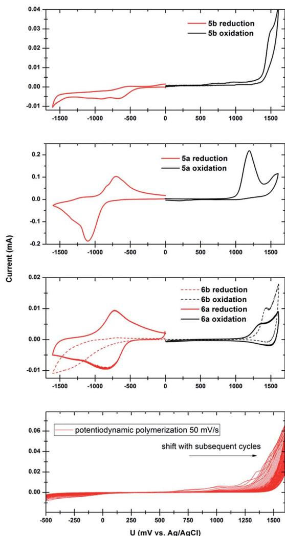
Fig. 4 Comparison of the cyclic voltammograms of **5b** measured in solution, **5a** measured as a film, and polymers **6a** and **6b** as films. A scan rate of 20 mV s<sup>-1</sup> was used in all cases. The bottom graph shows the potentiodynamic electropolymerization procedure for **5b** → **6b**.
