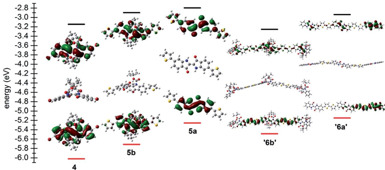
Fig. 3 Optimised ground-state geometries and frontier orbital energies of compounds 4, and 5a,b and cut-out segments of polymers 6a and 6b obtained by DFT calculations.
