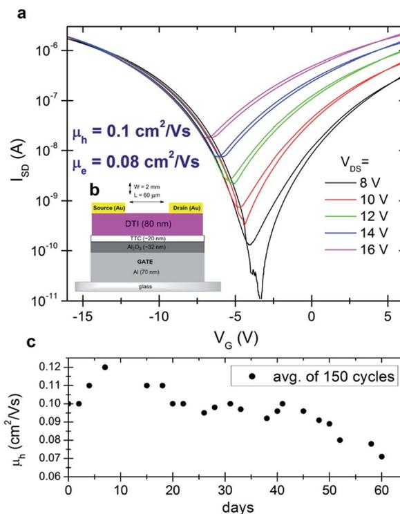
Fig. 6 DTI (**5a**) OFET transfer characteristics (a) with the inset (b) showing the device architecture used for the measurement. (c) OFET device lifetime study – mobility as a function of measurement days in air. Each day 150 cycles were applied.
