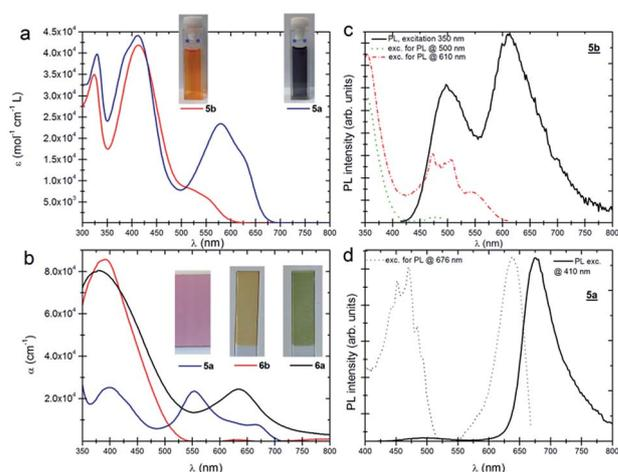
**Fig. 2** (a) UV-Vis absorption of **5a,b** in DMSO solution. Cuvettes show 0.1 mM solutions. (b) UV-Vis absorption of thin films on ITO glass. (c) Photoluminescence and excitation spectra of **5b** in DMSO solution. (d) Photoluminescence and excitation spectra of **5a** in DMSO.
