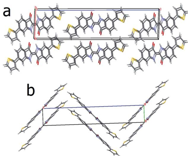
**Fig. 1** Crystal structure of DTI (**5a**). (a) A slightly tilted view down the *b*-axis, showing  $\pi$ - $\pi$  stacking interactions between H-bonded chains of indigos. (b) View down the *a*-axis, showing the direction of propagation of the H-bonded linear chains.
