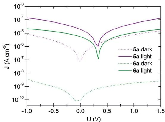
Fig. 7  $J$ - $V$  characteristics of ITO/DTI or poly(DTI)/Al devices, measured in the dark or under simulated solar illumination with an intensity of  $80 \text{ mW cm}^{-2}$ .
