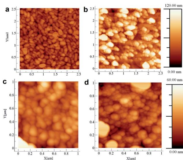
Fig. 5 AFM micrographs of (a) 80 nm of **5a** on ITO, (b) 80 nm of **5a** on AlO<sub>x</sub>/TTC, (c) a 140 nm film of **6b** polymerized on ITO, and (d) the same film after heating/deprotection, yielding **6a**.
