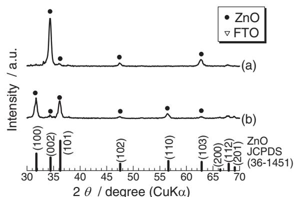
**Figure 4.** XRD  $2\theta$ -scan patterns of electrodeposited (a) ZnO/ZnO<sub>EY</sub> and (b) ZnO<sub>CA</sub>/ZnO<sub>EY</sub> bilayers.
