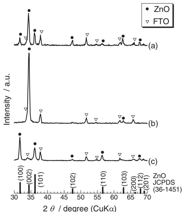
**Figure 2.** XRD  $2\theta$ -scan patterns of (a) pure ZnO, (b) ZnO<sub>EY</sub>, and (c) ZnO<sub>CA</sub> thin films electrodeposited on FTO glass substrates.
