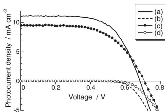
**Figure 8.** I-V curves of DSSCs employing (a, b) ZnO/ZnO<sub>EY</sub> and (c, d) ZnO<sub>CA</sub>/ZnO<sub>EY</sub> bilayer photoelectrodes sensitized with D149 measured under illumination with (a, c) an AM 1.5 stimulated sunlight (100 mW cm<sup>-2</sup>) and (b, d) in the dark.
