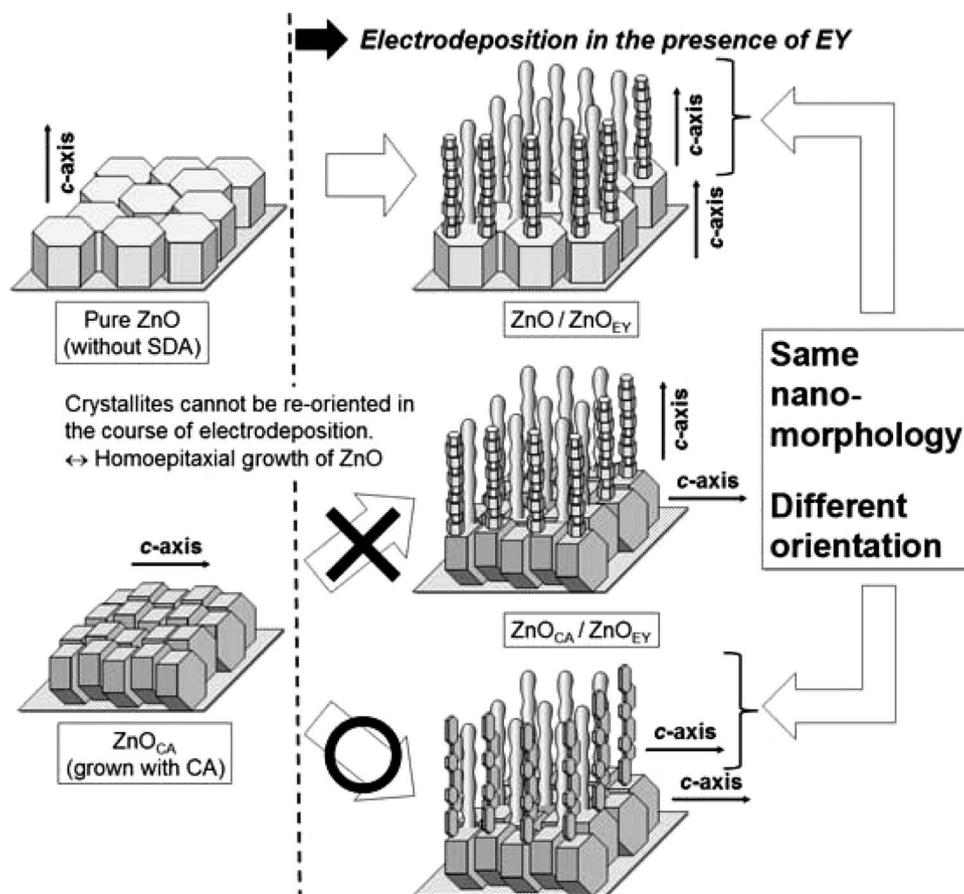
**Figure 6.** Illustration of the bilayer electrodeposition by switching SDA in the course of the electrodeposition of ZnO.
