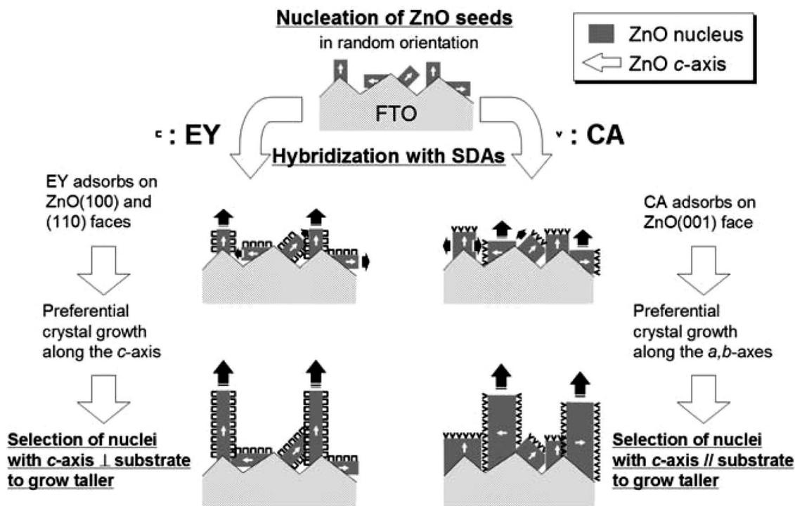
**Figure 5.** Illustration of the mechanism that cause different crystallographic orientations of the ZnO hybrid thin films with EY and CA, based on the selection of preferentially growing ZnO nuclei.
