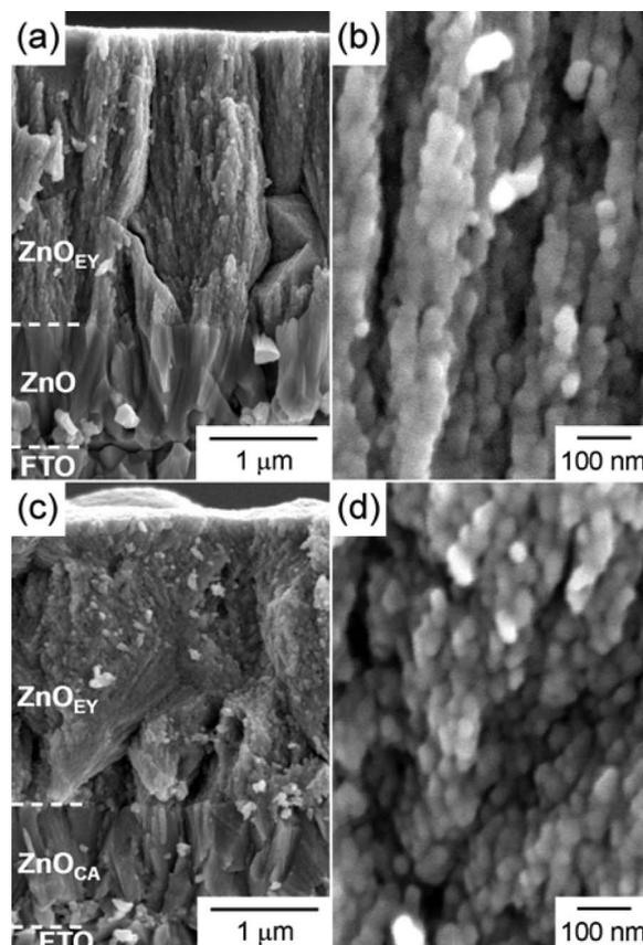
**Figure 3.** Cross-sectional SEM images of electrodeposited (a, b) ZnO/ZnO<sub>EY</sub> and (c, d) ZnO<sub>CA</sub>/ZnO<sub>EY</sub> bilayers, where (b) and (d) correspond to the close-up of the ZnO<sub>EY</sub> outer layer to show their nanostructures, respectively.
