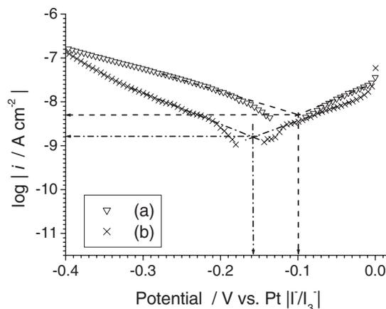
**Figure 9.** Tafel plots of I-V curves measured at (a) ZnO and (b) ZnO<sub>CA</sub> electrodes in I<sub>3</sub><sup>-</sup> redox electrolyte.
