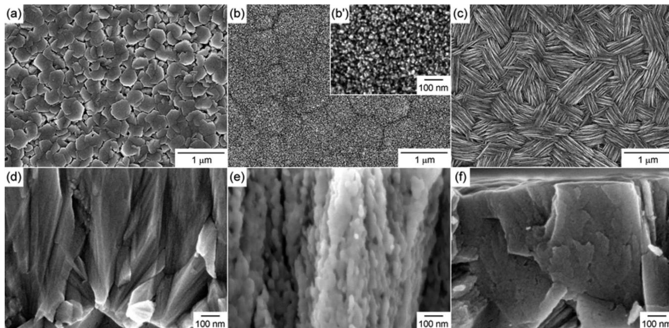
**Figure 1.** Surface and cross-sectional SEM pictures of electrodeposited (a, d) pure ZnO, (b, b', e) ZnO<sub>EY</sub> and (c, f) ZnO<sub>CA</sub> thin films obtained after desorption of the loaded organic molecules.
