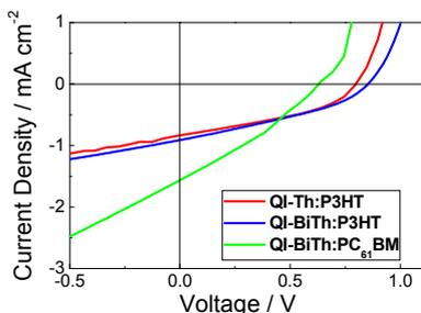
**Figure 3.** Current density-voltage curves of OPV devices based on QI derivatives under AM 1.5 G.
