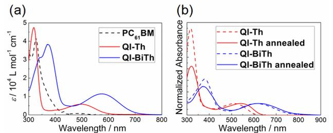
**Figure 2.** UV-vis absorption spectra of QI derivatives (a) in CHCl<sub>3</sub> and (b) in spin-coated film (normalized by absorbance at the top of band correspond to the  $\pi-\pi^*$  transition, dot line: as-cast films, solid line: annealed films at 100 °C for 10 min).
