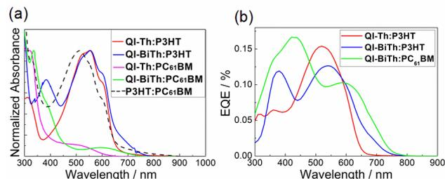
**Figure 4.** (a) UV-vis absorption spectra of active layers based on QI derivatives. (b) EQE spectra of the OPV devices based on QI derivatives.
