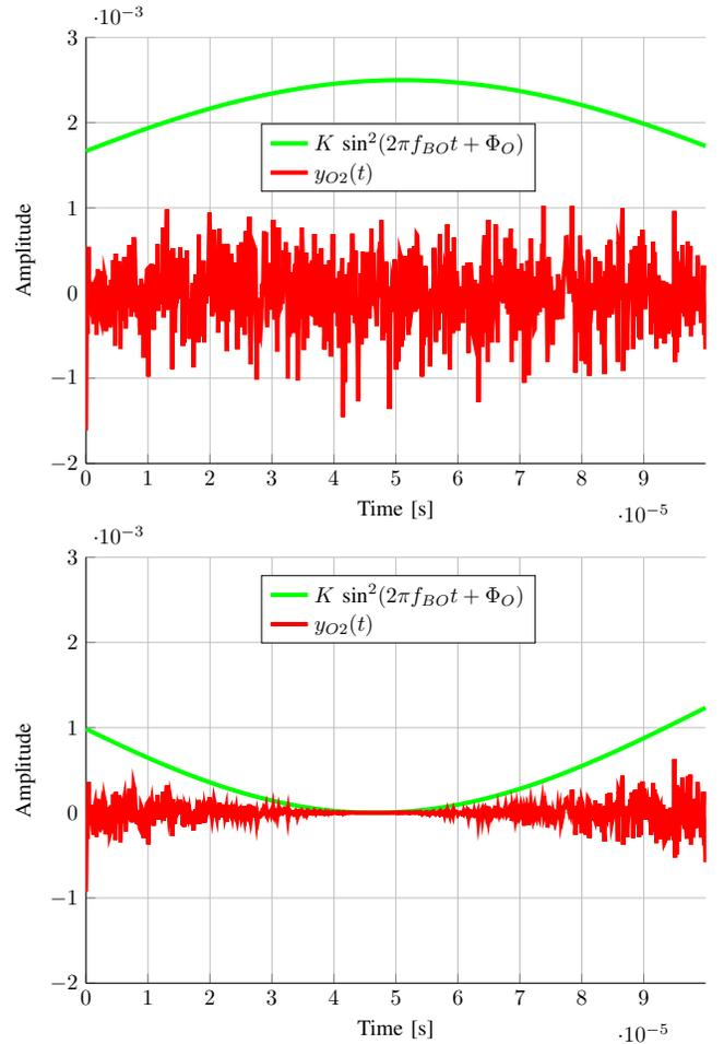
Fig. 2. OCT IF signal terms  $K \sin^2(2\pi f_{BO}t + \Phi_O)$  and  $y_{O2}(t)$  for  $\tau_O = 192$  ps (upper plot) and  $\tau_O = 232$  ps (lower plot).
