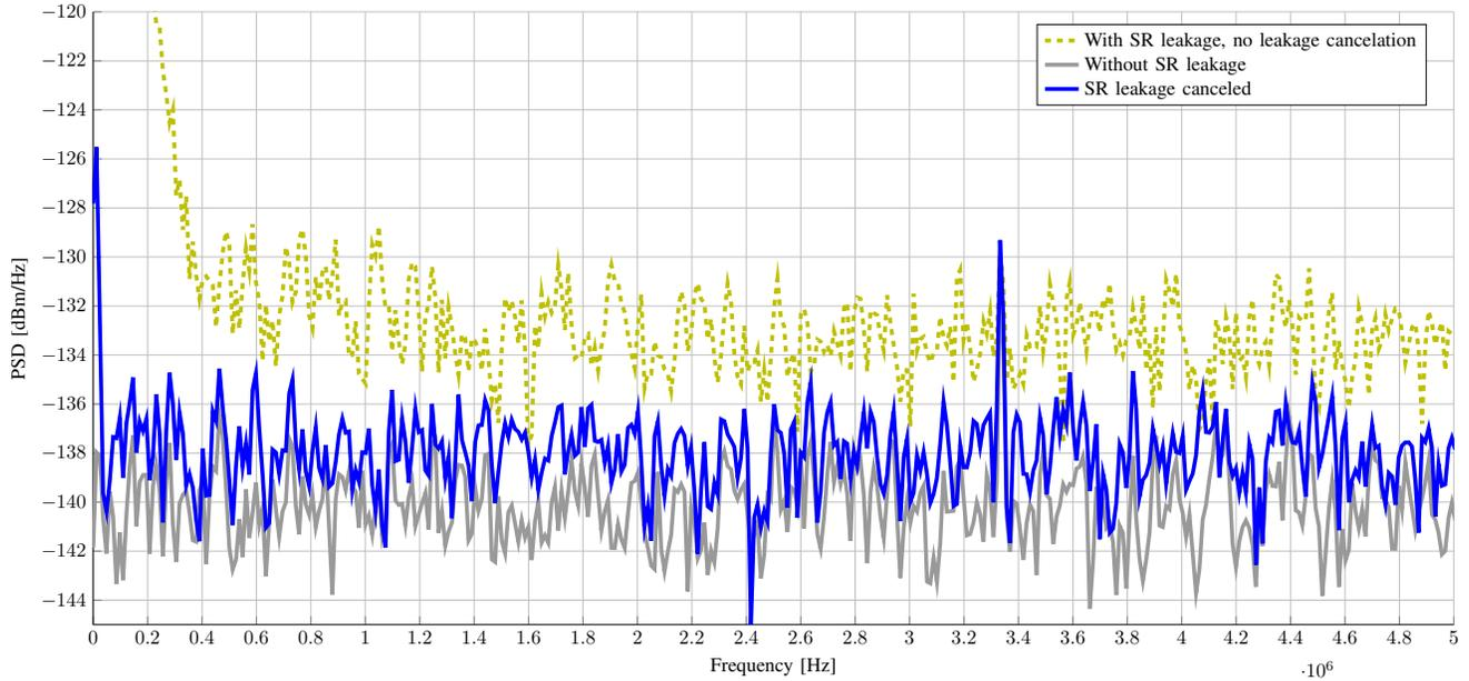
Fig. 3. Estimation of the IF PSD with/without SR leakage. It can be observed that with the SR leakage the sensitivity of the system is degraded notably. However, with the extracted DPN from the OCT, the SR leakage can be suppressed significantly and ultimately the target in the channel is recovered well.
