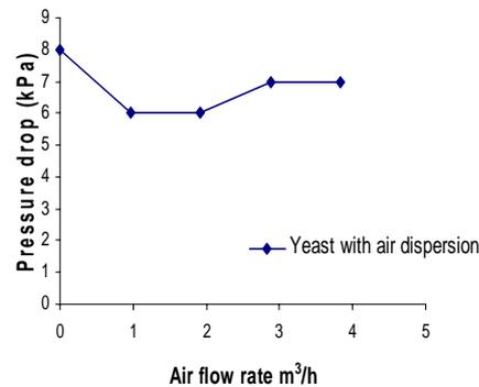
Fig-8 Effect of air dispersion on pressure drop; feed flow rate=2m<sup>3</sup>/h; Inlet pressure= 0,7bar
