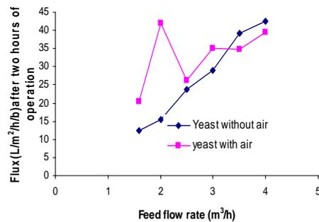
Fig-5 Effect of feed flow rate on the permeate flux. TMP =0,7bar; Air flow rate = 2,88 m<sup>3</sup>/h; Yeast concentration = 6,1g/L (dry-mass); pH=5,5
