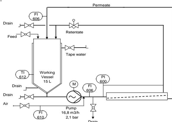
Fig-2 Schematic diagram of experimental set up for microfiltration
