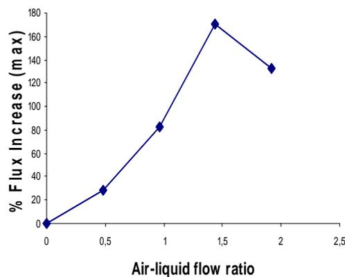
Fig-4 Effect of air-liquid ratio on percent permeate flux enhancement. TMP =0,7bar; Feed flow rate = 2m<sup>3</sup>/h; Yeast concentration = 6,1g/L (dry-mass); pH=5,5
