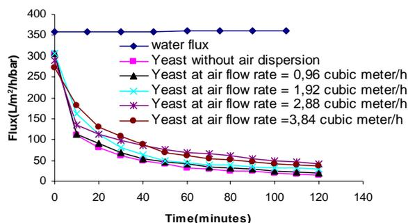
Fig-3 Effect of two-phase air-liquid flow on the permeate flux. TMP = 0,7bar; Feed flow rate = 2m<sup>3</sup>/h; Yeast concentration = 6,1g/L (dry-mass); pH=5,5
