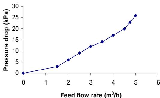
Fig-7 Effect of feed flow rate on pressure drop This drop in pressure is major draw back of running a microfiltration process at high liquid
