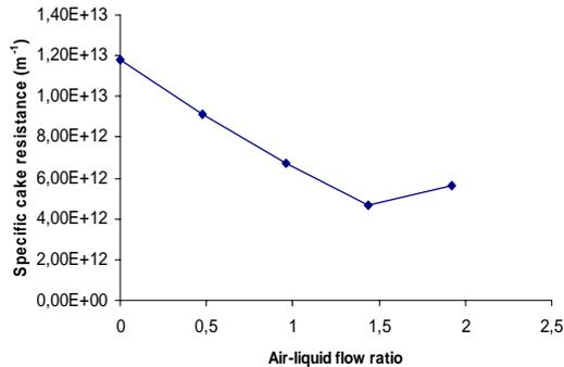
Fig-6 Effect of air-liquid ratio on specific cake layer resistance; TMP =0,7bar; Feed flow rate = 2m<sup>3</sup>/h; Yeast concentration = 6,1g/L (dry-mass); pH=5,5
