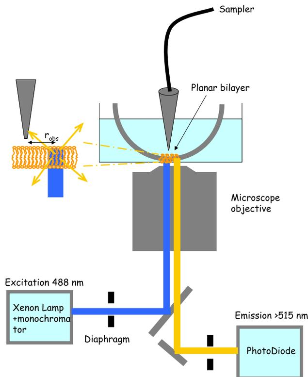
**Fig. 1** Scheme of the experimental setup. Horizontal planar bilayers were formed in a chamber placed in a fluorescent microscope. The shift in local pH was carried out by microinjection using micropipette connected to a sampler. The fluorescence from the observation area was collected by a system of diaphragms
