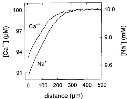
FIGURE 2 Representative calcium and sodium concentration profiles at the *cis* side of a BLM. By using a double-barreled microelectrode they were recorded simultaneously. Due to the addition of 0.3 M choline chloride at the *cis* side a transmembrane volume flux was induced. The bulk solution contained 10 mM Tris, 10 mM Mes, 10 mM NaCl, and 0.1 mM  $\text{CaCl}_2$ . The  $\text{Na}^+$  and  $\text{Ca}^{2+}$  USL thicknesses were, respectively, 130 and 105  $\mu\text{m}$ .
