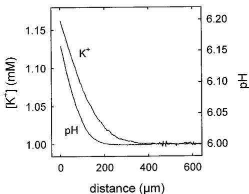
FIGURE 4 Simultaneously measured  $K^+$  concentration and pH profiles. The aqueous solutions contained 1 (1) mM Mes, 0.1 (0.1) M choline chloride, and 1 (10) mM KCl at the *trans* (*cis*) side of the BLM. Nigericin was added to the *cis* side in a final concentration of 16  $\mu\text{M}$ . The USLs found for  $K^+$  and pH (108 and 67  $\mu\text{m}$ , respectively) are very different in size.
