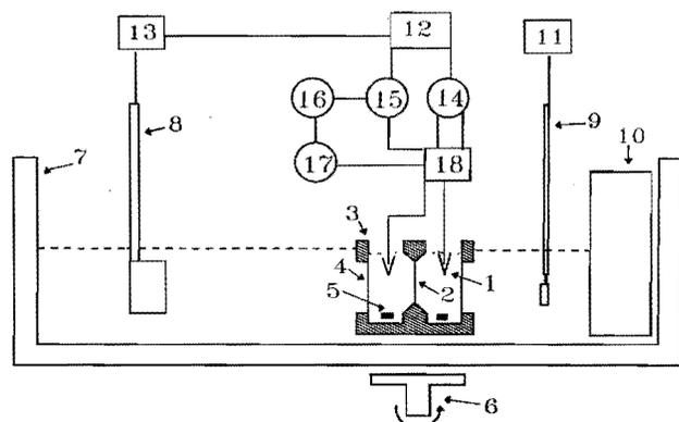
Fig. 1. Scheme of the experimental arrangement. 1, Reference electrodes; 2, bilayer lipid membrane; 3, teflon support; 4, acoustic window; 5, magnetic stirrer bar; 6, stirrer; 7, water bath; 8, ultrasound transducer; 9, ceramic hydrophone; 10, absorber; 11, selective nanovoltmeter; 12, personal computer; 13, rf generator; 14, electrometer; 15, current amplifier; 16, oscilloscope; 17, triangle wave generator; 18, switch: connects the electrodes either to 14 or to 15 and 17.
