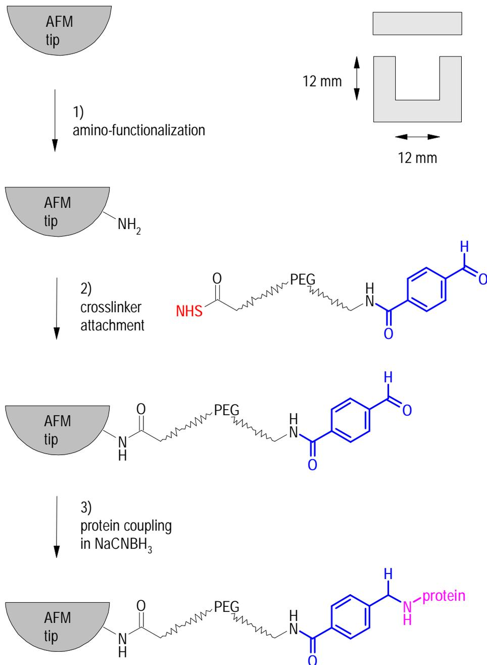
**Figure 2:** Reaction of amino-functionalized AFM tips with Aldehyde-PEG-NHS and subsequent coupling of protein. Please, note that coupling is performed in sodium cyanoborohydride which converts the initially formed C=N bond into a stable C-N bond.
