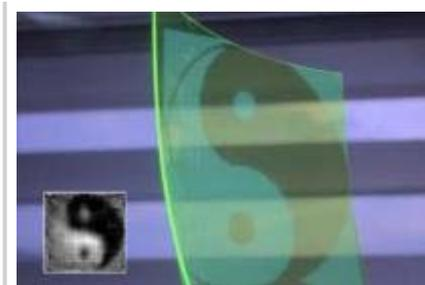
This shows a comparison between the (ground truth) image being focused on the sensor surface and the reconstructed image (inset). Credit: Photo courtesy Oliver Bimber, Johannes Kepler University Linz.
