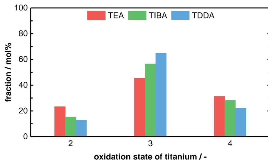
Figure 4: Comparison of the titanium oxidation states for different alkyls.
