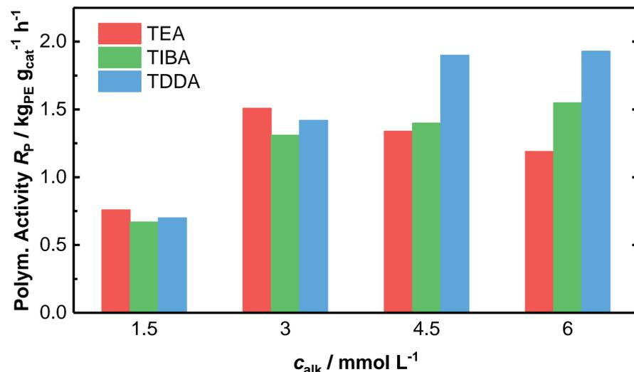
Figure 3: Polymerization activity for different alkyls and their respective concentration.
