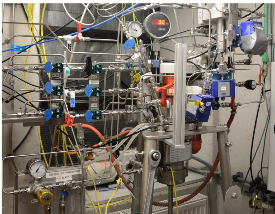
Figure 2: The polymerization experiments were carried out in a 0.5 L reactor system.
