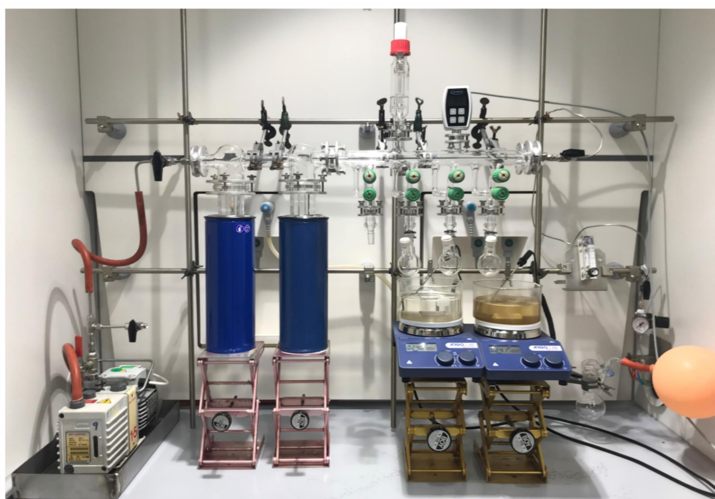
Figure 3: Schlenk apparatus used for unimpeded polymerization tests.
