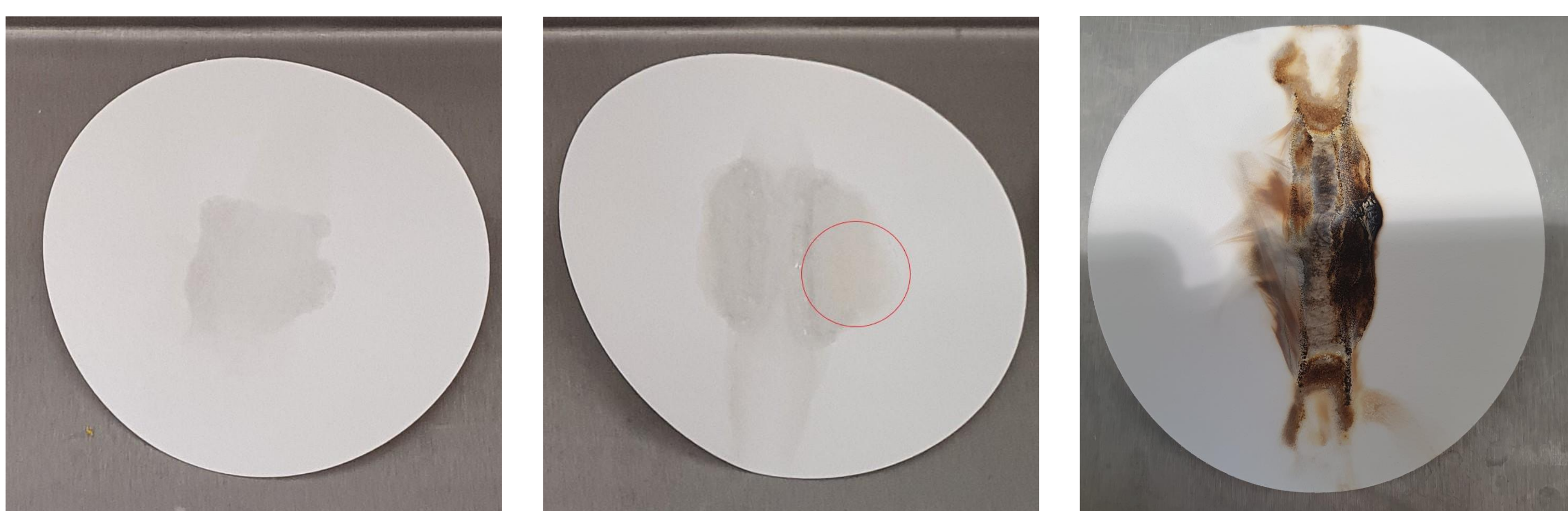
Figure 1: left: Pyrophoricity test with a solution of a 30 wt.% of the ionic liquid in n -heptane. middle: Pyrophoricity test with a solution of a 40 wt.% of the ionic liquid in n -heptane. right: Pyrophoricity test with the pure ionic liquid.
