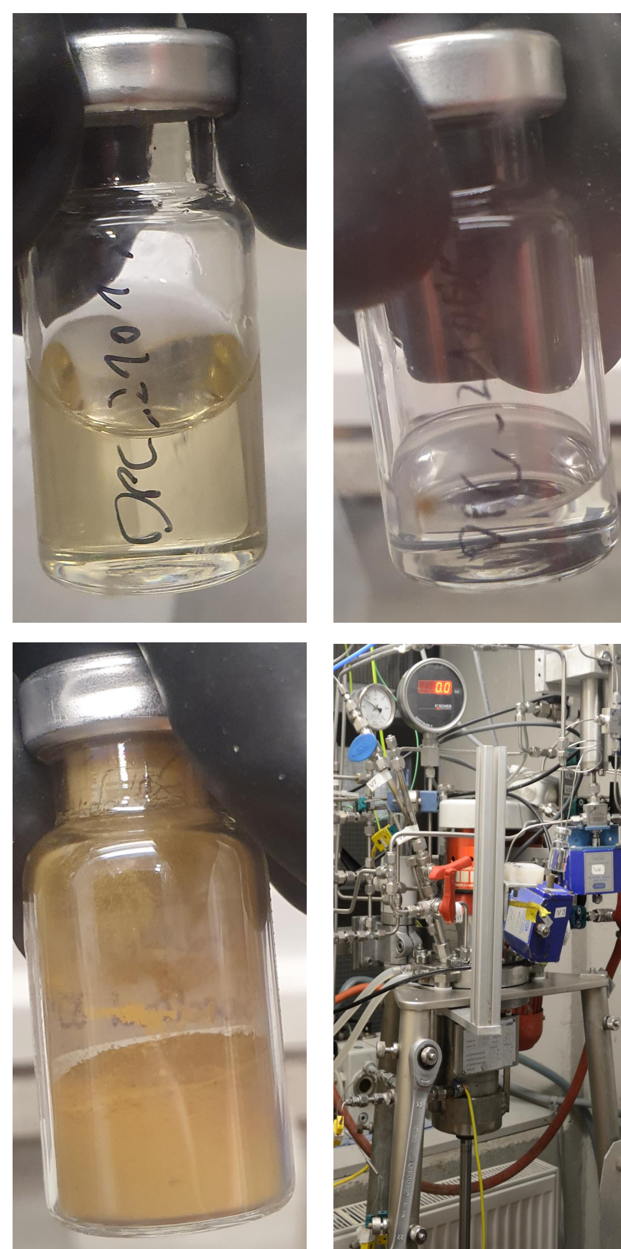
Figure 2: top left: IL with NMeOct 3 Cl at the ratio 5. top right: Mg-Al-alkyl with the ratio 2. bottom left: ZN catalyst with 7.4 wt.% Ti. bottom right: 0.5 L polymerization reactor.
