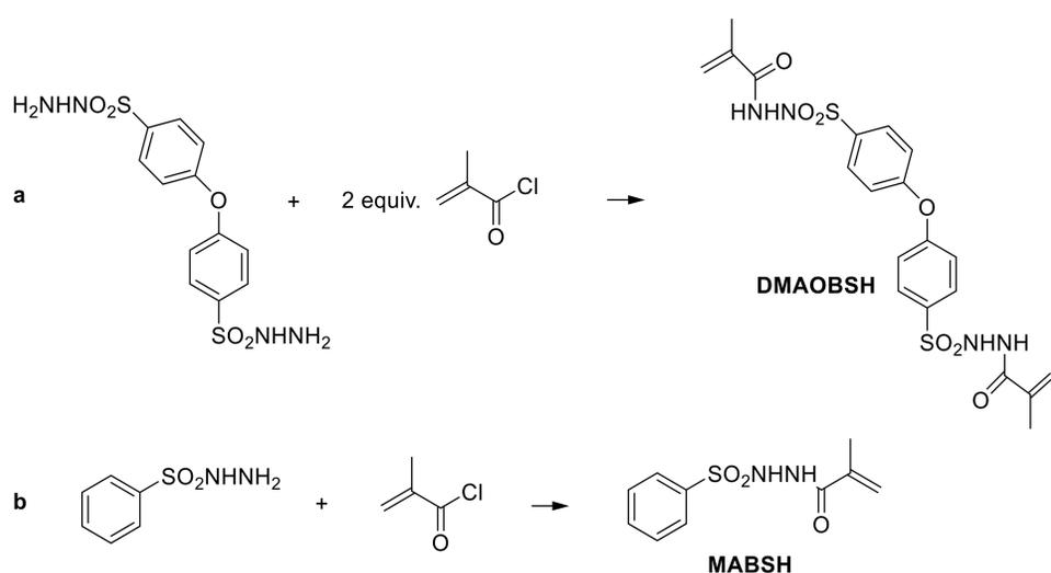
Figure 1: Modification of OBSH (a) and BSH (b).
