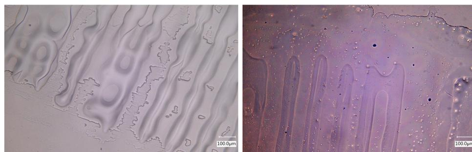
Figure 3: Printed layer before (left) and after (right) the foaming step.
