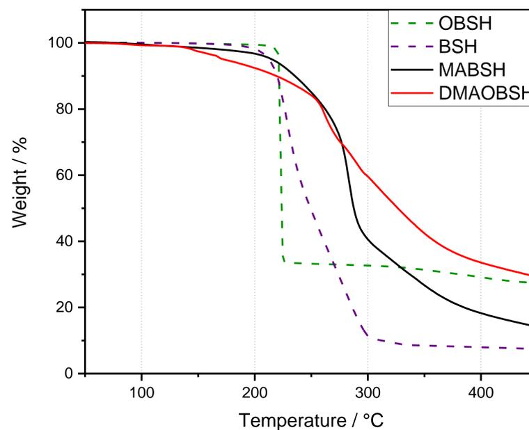
Figure 2: Comparison of the TGA analysis of OBSH, BSH, MABSH and DMAOBSH.
