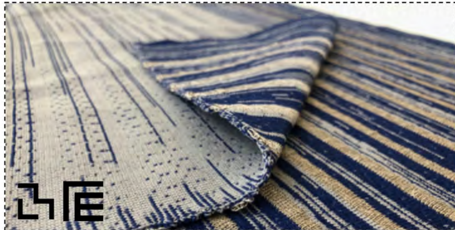
Responsive fabric with multi-layer pressure sensing matrix
