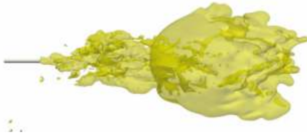
Fig.3: Interface-resolved simulation of supersonic air injection into liquid in the near-nozzle region using the compressible VOF method and large eddy simulation.
