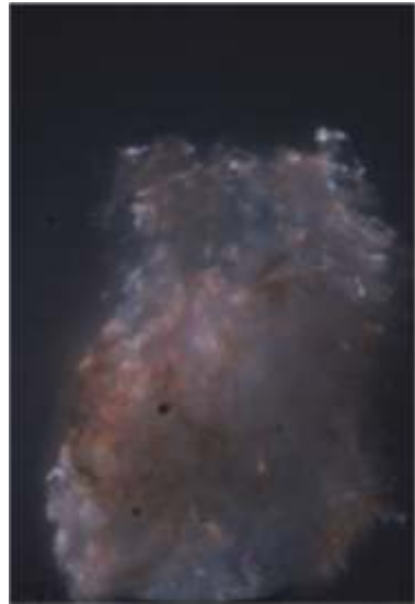
Fig.2: The same experiment a few milliseconds later recorded with a second camera running at extremely low exposure time per frame to show the flame structure.
