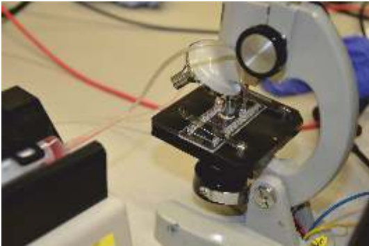
Fig.1: Seminar 2012 Bloody Fluid Dynamics: This is how we observed our own red blood cells flow through a channel.
