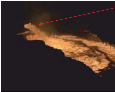
Fig.1: Taphole recorded with a camera in the visual range (left) and the infrared spectrum (right) (images from voestalpine).
