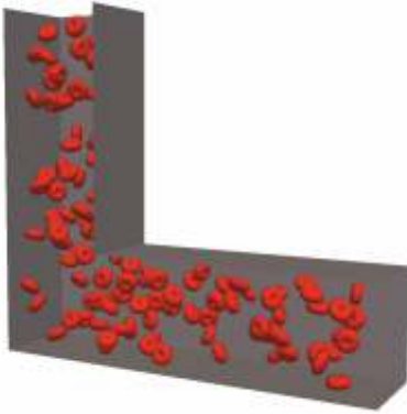
Fig.1: Resolved simulation of red blood cells in different microfluidic conditions using the immersed-boundary method coupled with a reduced-order RBC model.
