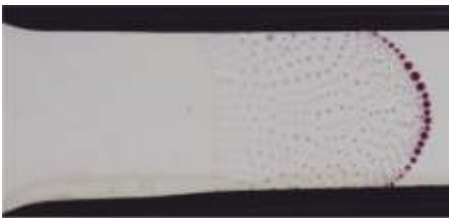
Fig.3: Droplet moving along a lateral channel in laminar flow. Coalescence of droplets at the flow front forms a characteristic size range that depends on the alcohol concentration.
