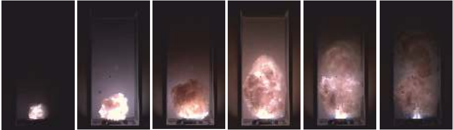
Fig.1: Image series of a dust deflagration experiment for 5g of aluminum powder recorded at extremely low exposure times. Metallic dusts show a much brighter flame compared to organic dust deflagration (cf. last year's annual report).
