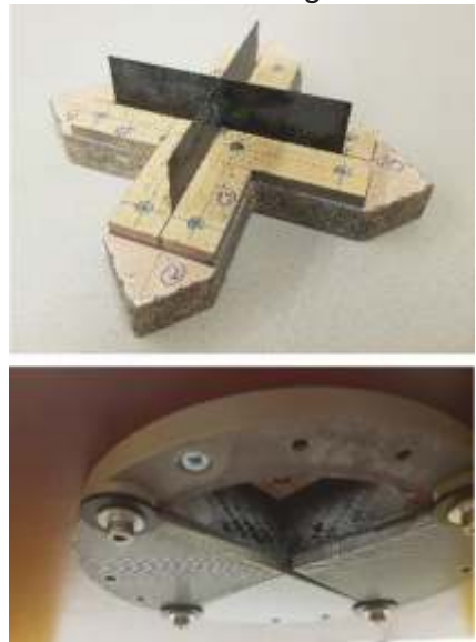
Fig.2: Stencil and die bottom. The stencil used to split the material and the bottom to empty the die quarters separate.
