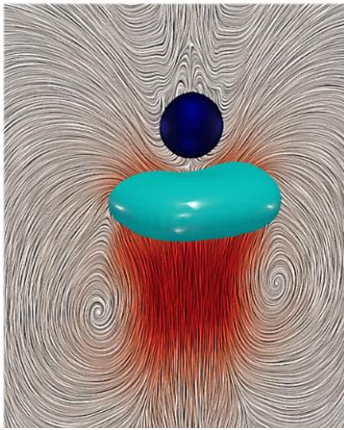
VOF-IB simulation of a rising bubble and a falling particle in a water column.
