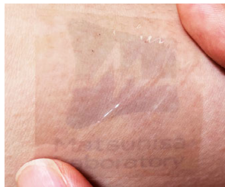
Figure 1: Transparent and stretchable polymer conductors patterned by UV laser ablation.
