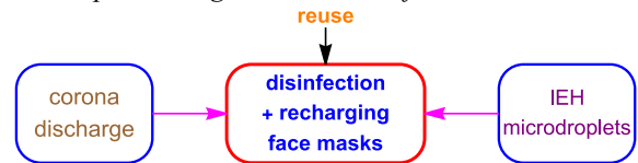
Fig. 3 Disposed face masks can be recharged either by corona charging or IEH microdroplet charging. Interestingly, these processes can be invoked for disinfection as well, because both are chemically reactive.
