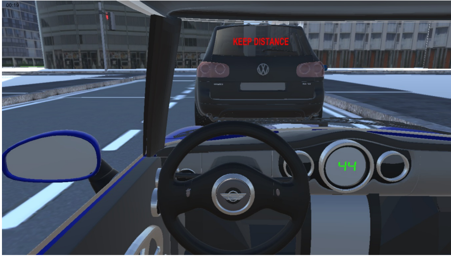
Fig. 4. Windshield-conveyed message related to safety distance, independent of the communication capabilities of the trailing vehicle (adapted from [43]).
