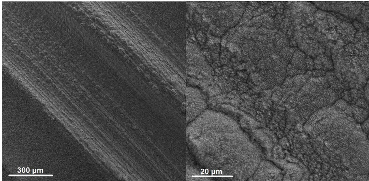
**Fig. 3:** SEM images of laser-induced ring on sand-blasted titanium dental screw. The left image shows an overview of the laser-induced structures on the screw, where only a few micro-sized bumps can be seen. At a higher magnification (right image) the nano-sized ripples are visible.
