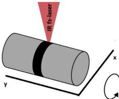
**Fig. 1:** Schematics of continuous laser processing of cylindrical samples. The laser is focused onto the highest point of the cylindrical sample. For continuous laser processing, the sample is irradiated while being rotated and moved along the  $y$ -axis, leading to a spiral around the cylinder. Figure adapted from [1].
