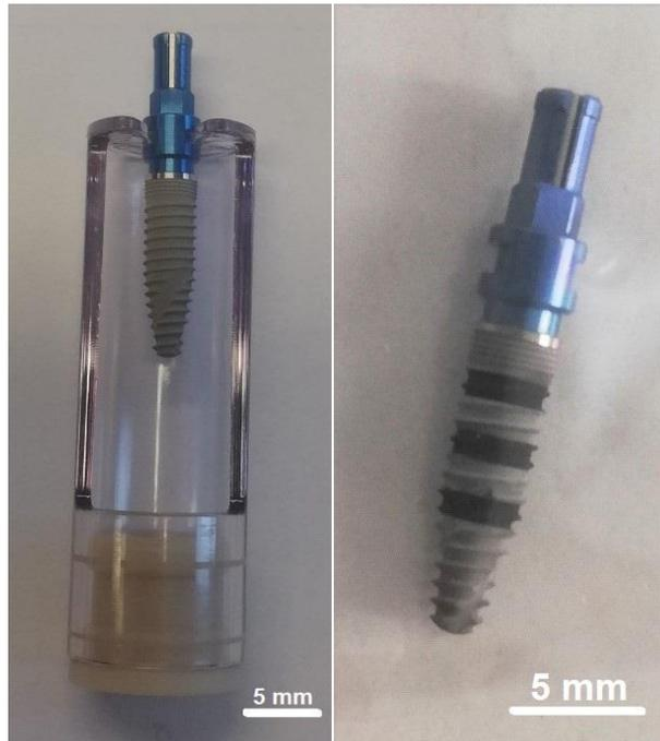
**Fig. 2:** Images of unprocessed dental screw (left image, in casing) and laser-treated dental screw in 3 rings in black (right image).
