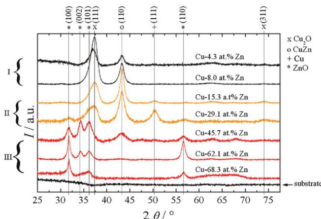
**Figure 6** XRD spectra of selected compositions on the surface of the Cu–Zn thin film oxide alloy library.
