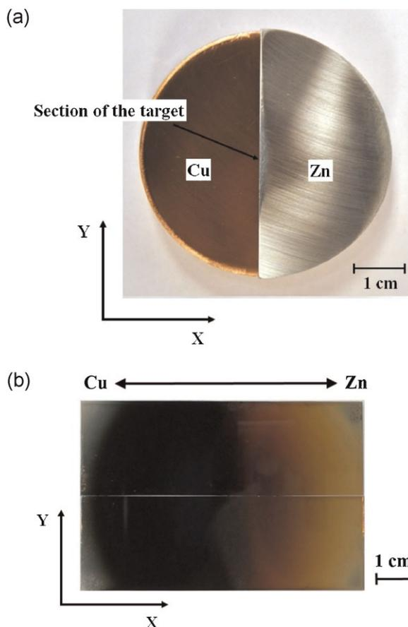
**Figure 1** (a) Two-component sectioned metallic Cu–Zn target. (b) Photograph of the as-deposited film on a double glass substrate.
