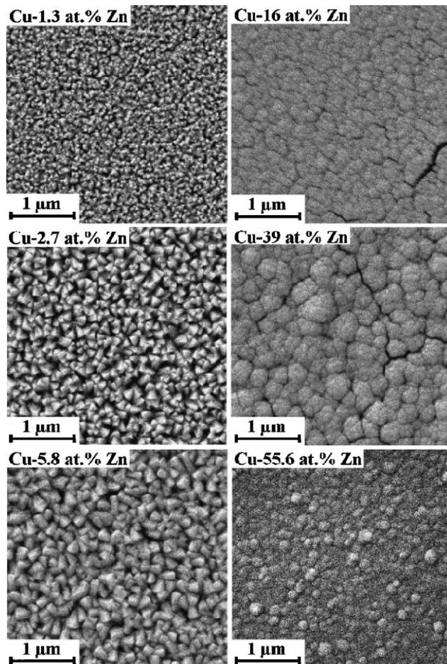
**Figure 4** SEM image of the Cu–Zn combinatorial library on various positions on the sample.
