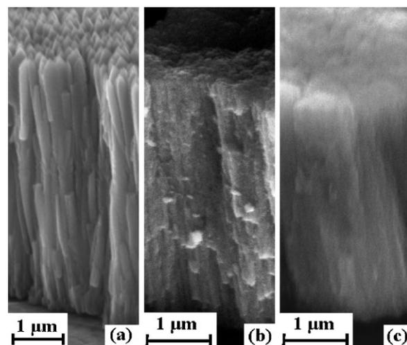
**Figure 5** SEM image of the cross-section of the Cu–Zn thin film oxide alloys for various compositions, (a) Cu–1.5 at.% Zn, (b) Cu–25.4 at.% Zn, and (c) Cu–53.7 at.% Zn.
