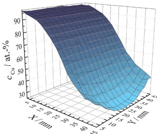
**Figure 2** Scanning XRF analysis map of the Cu–Zn thin film oxide alloy obtained by sectioned target co-sputter deposition.
