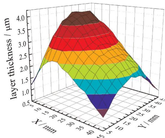
**Figure 3** Distribution of the Cu–Zn thin film oxide alloy thickness with respect to the position on the sample.
