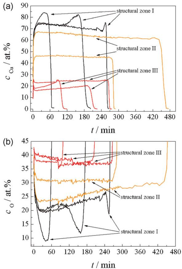
**Figure 7** (a) XPS depth profile of the Cu–Zn thin film oxide alloys for various compositions showing the in-depth Cu concentration depending on the XPS sputter time  $t$ . (b) XPS depth profile of the Cu–Zn thin film oxide alloys for various compositions showing the in-depth O concentration depending on the XPS sputter time  $t$ .
