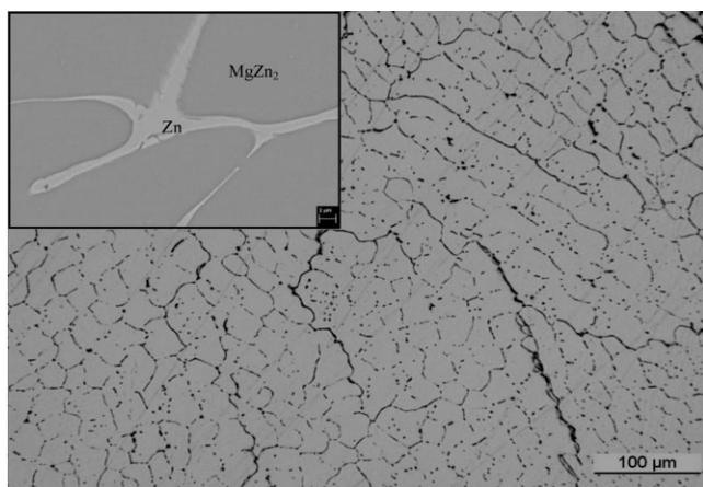
**Figure 3** Optical micrograph and SEM image (inset) of a MgZn<sub>2</sub> sample.
