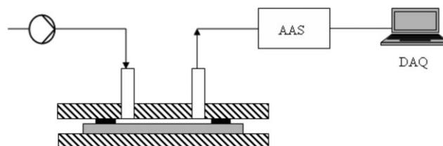
**Figure 2** Experimental setup for flow experiments. Arrows indicate the electrolyte flow through the cell.
