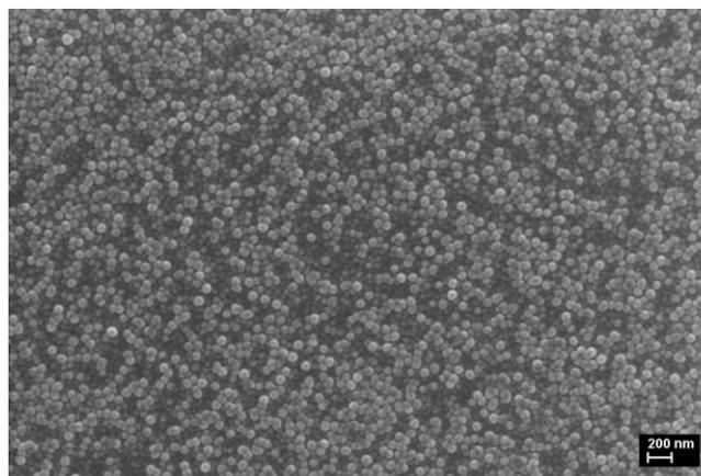
**Figure 6** SEM micrograph of a thermally evaporated Mg–27.1 at.% Zn sample.
