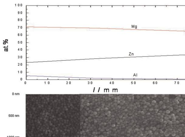
**Figure 7** EDX analysis results and SEM images of an  $\text{Al}$ – $\text{Mg}$ – $\text{Zn}$  thin film.
