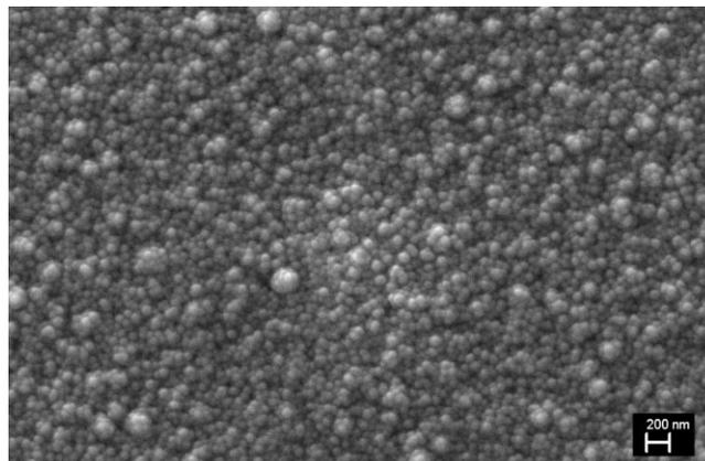
**Figure 5** SEM micrograph of a thermally evaporated MgZn<sub>2</sub> sample.
