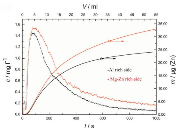
**Figure 8** (online colour at: [www.pss-a.com](http://www.pss-a.com)) Dissolution curves of an Al–Mg–Zn thin film at different positions on the sample surface.
