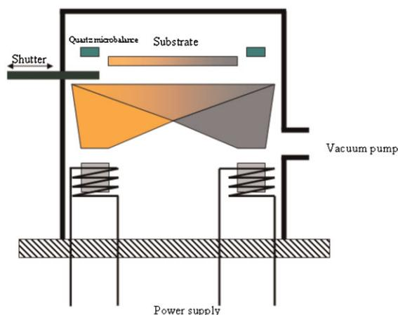
**Figure 1** (online colour at: www.pss-a.com) Evaporation setup for co-evaporation of Mg–Zn and Al bulk material sources.
