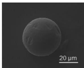
**Figure 4** SEM image of a micro sphere on the sample surface.
