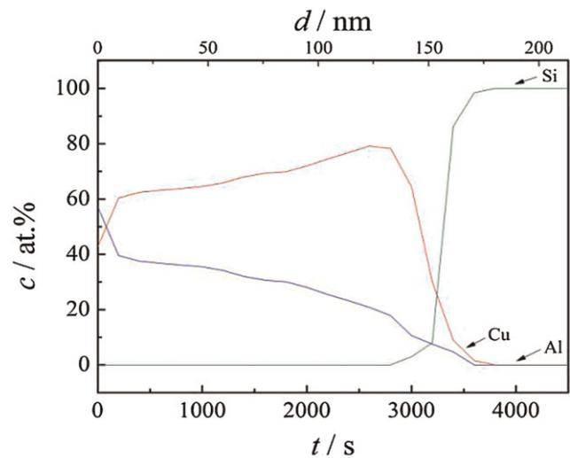
**Figure 4** XPS depth profiles of Al–Cu thin films evaporated from two different sources.
