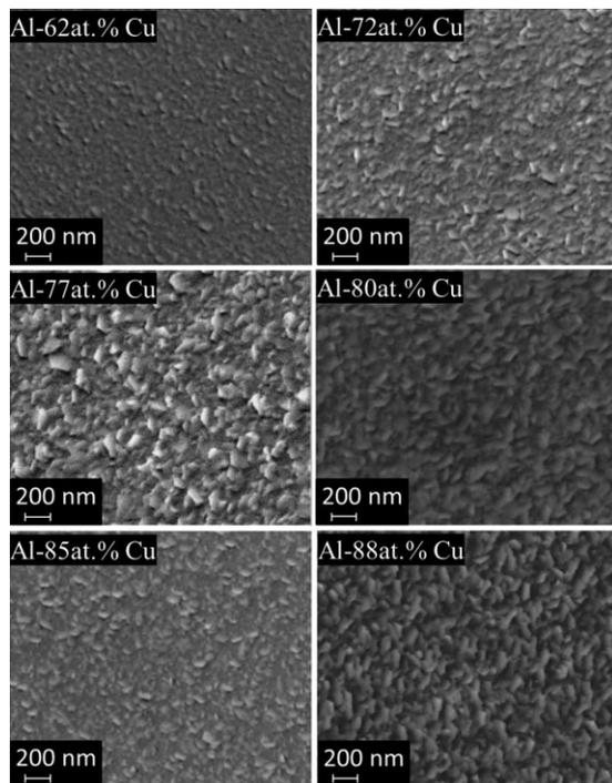
**Figure 2** SEM image of Al–Cu thin film library evaporated from two sources.
