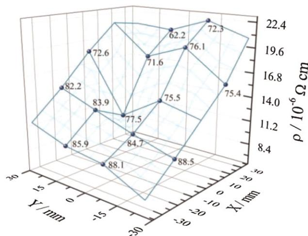
**Figure 5** Electrical resistivity of Al–Cu thin films deposited from dual sources. The Cu content (at.%) is given for each point.
