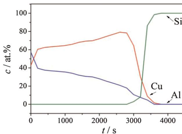
**Figure 7** XPS depth profiles of Al–Cu thin film evaporated from a single source.
