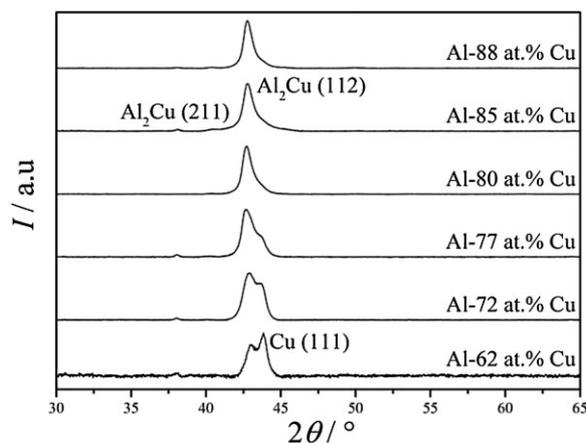
**Figure 3** XRD results of Al–Cu thin films co-deposited from two different sources.
