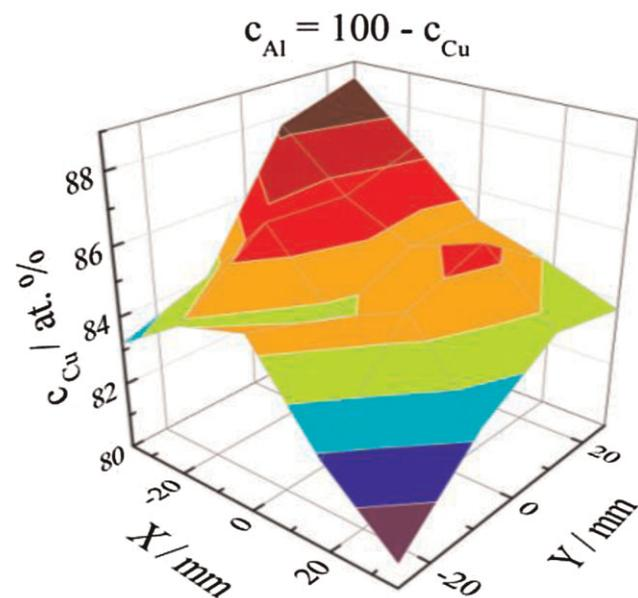
**Figure 6** EDX of Al–Cu thin film alloys evaporated from a single sources.
