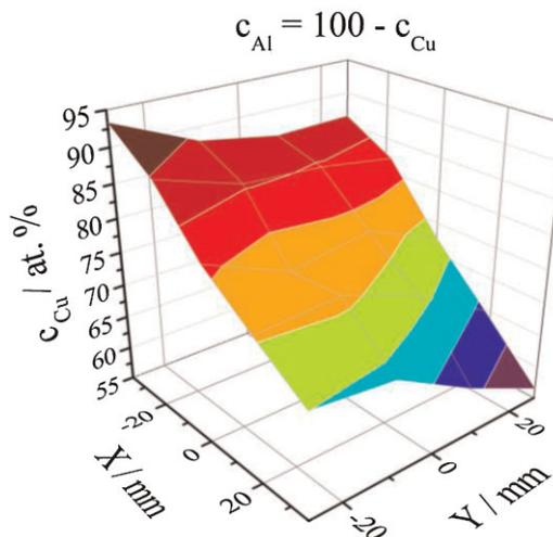
**Figure 1** EDX of Al–Cu thin film compositional spread evaporated from two individual sources.
