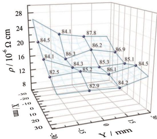
**Figure 8** Electrical resistivity of Al–Cu thin films deposited from alloy source. The Cu content (at.%) is given for each point.
