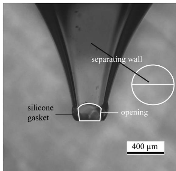
Fig. 1. Optical image of the capillary tip, side view, perpendicular to the plane of the separating wall.
