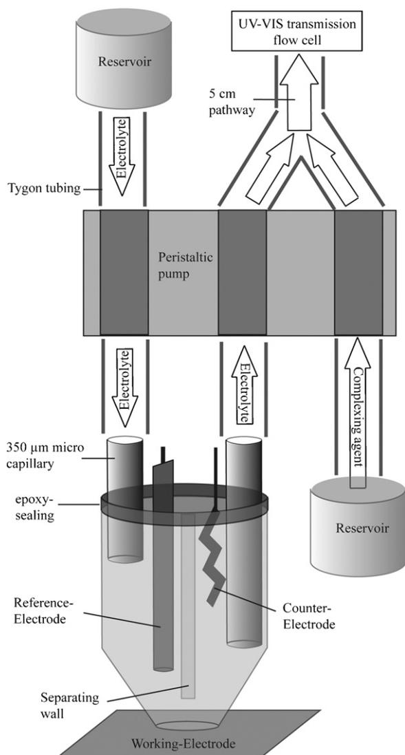
Fig. 2. Schematic drawing of the flow type scanning droplet cell.
