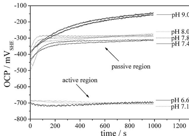
**Fig. 5.** Corrosion potential transients of pure zinc in 0.1 M borate buffer at different pH values.
