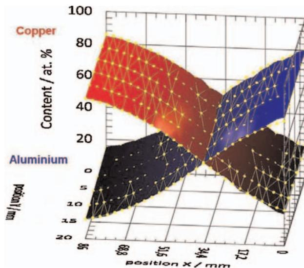
**Figure 6** (online color at: [www.pss-a.com](http://www.pss-a.com)) A binary Cu–Al gradient (colored surface plot) with model fit (yellow spheres/lines, see text).
