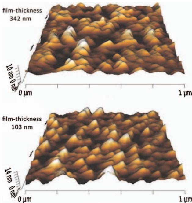
**Figure 3** (online color at: www.pss-a.com) 3D AFM images ( $1 \times 1 \mu\text{m}^2$ , Z-range 10 and 14 nm) of the copper film at different spots.
