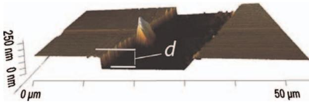
**Figure 2** (online color at: www.pss-a.com) AFM 3D topography image over a cut showing the thickness  $d$ .
