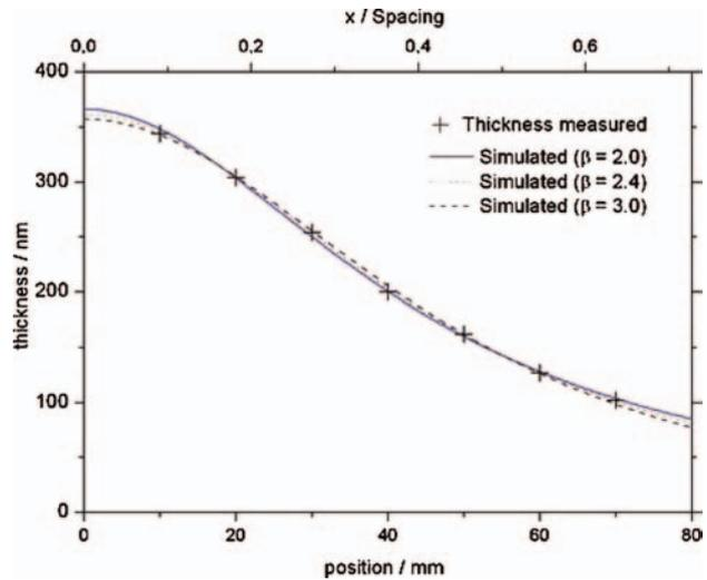
**Figure 4** (online color at: www.pss-a.com) Measured film thickness of pure copper from a single evaporation source.
