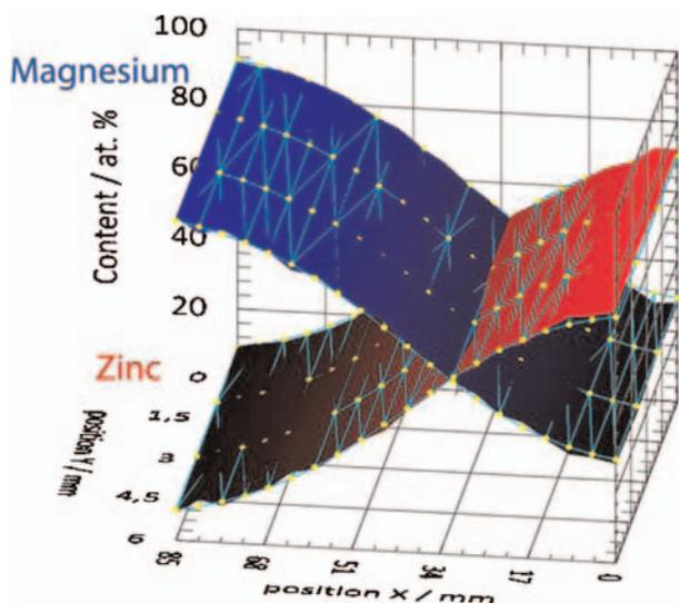
**Figure 7** (online color at: [www.pss-a.com](http://www.pss-a.com)) A binary Zn–Mg gradient with model fit.
