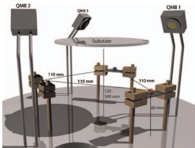
**Figure 1** (online color at: [www.pss-a.com](http://www.pss-a.com)) Schematic illustration of the PVD geometry.
