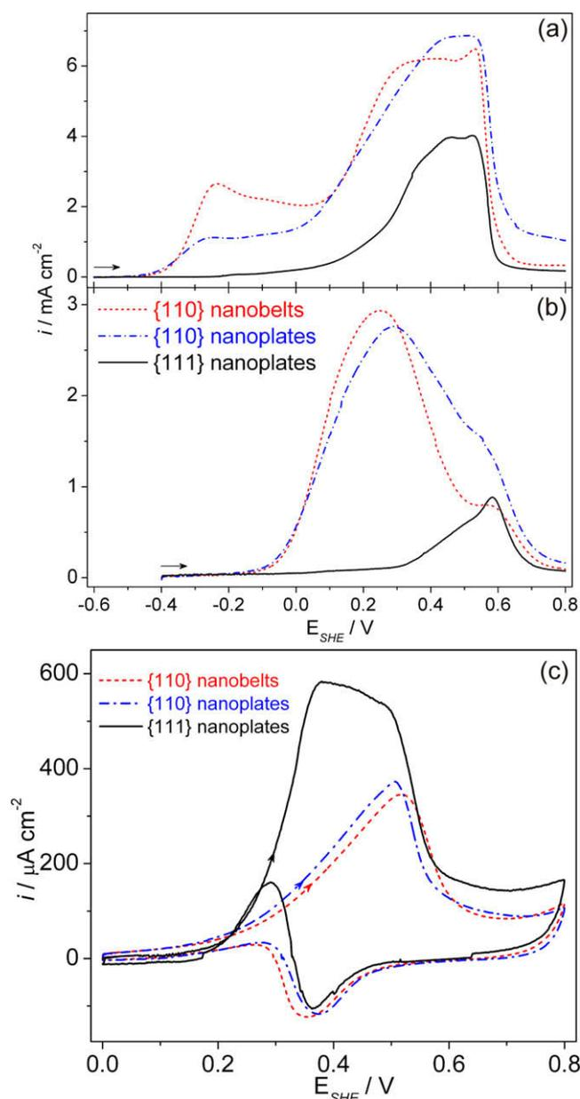
**Fig. 2.** Typical voltammetric curves of {1 1 0} Au nanobelts, {1 1 0} nanoplates and {1 1 1} nanoplates in (a) 0.1 M NaOH with 10 mM glucose, (b) phosphate buffer (pH = 7.4) with 10 mM glucose, and (c) 0.1 M NaOH with 1.5 M CH<sub>3</sub>OH, respectively. Scan rate: 20 mV/s.
