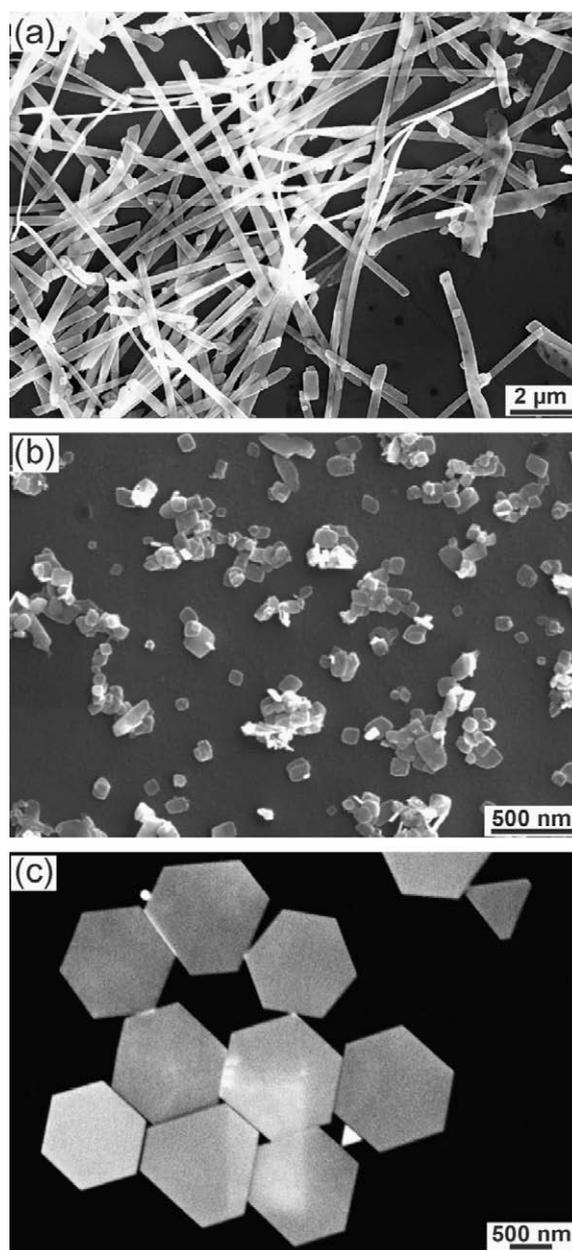
Fig. 1. FE-SEM images of (a) Au nanobelts, (b)  $\{110\}$  Au nanoplates with a square shape and (c)  $\{111\}$  Au nanoplates with hexagonal shape.
