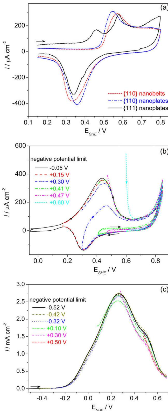
**Fig. 3.** (a) Cyclic voltammograms of {1 1 0} Au nanobelts, {1 1 0} nanoplates and {1 1 1} nanoplates in 0.1 M NaOH solution without the presence of CH<sub>3</sub>OH. (b) Cyclic voltammograms of {1 1 0} Au nanobelts in 0.1 M NaOH with 1.5 M CH<sub>3</sub>OH. (c) positive scan of cyclic voltammograms of {1 1 0} Au nanobelts in phosphate buffer (pH = 7.4) with 10 mM glucose with different negative potential limits. Scan rate: 20 mV/s.
