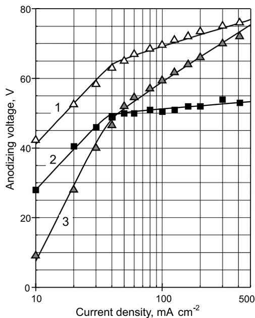
Fig. 3. Variation of anodizing voltage with current density for (1) steady-state aluminium anodizing in non-stirred  $0.4 \text{ mol dm}^{-3} \text{ H}_2\text{C}_2\text{O}_4$ , (2) for anodizing in non-stirred  $1.4 \text{ mmol dm}^{-3} \text{ NH}_4\text{F}$ ,  $0.4 \text{ mol dm}^{-3} \text{ H}_2\text{C}_2\text{O}_4$ , and (3) for anodizing in stirred  $1.4 \text{ mmol dm}^{-3} \text{ NH}_4\text{F}$ ,  $0.4 \text{ mol dm}^{-3} \text{ H}_2\text{C}_2\text{O}_4$ .
