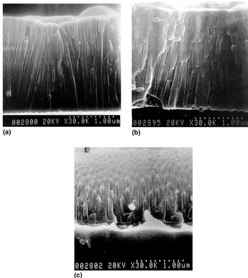
Fig. 4. Scanning electron micrographs of fracture-sections of porous oxide films formed by galvanostatic anodizing at  $10 \text{ mA cm}^{-2}$  for 7 min in (a)  $0.4 \text{ mol dm}^{-3} \text{ H}_2\text{C}_2\text{O}_4$  at 50 V, (b) non-stirred  $0.5 \text{ mmol dm}^{-3} \text{ NH}_4\text{F}$ ,  $0.4 \text{ mol dm}^{-3} \text{ H}_2\text{C}_2\text{O}_4$  at 38 V and (c) stirred  $2.5 \text{ mmol dm}^{-3} \text{ NH}_4\text{F}$ ,  $0.4 \text{ mol dm}^{-3} \text{ H}_2\text{C}_2\text{O}_4$  at 3 V.
