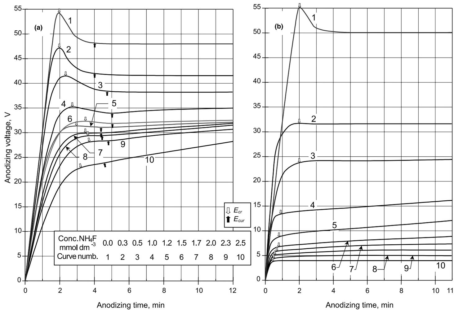
Fig. 1. Voltage–time responses for anodizing aluminium at a constant current density of  $10 \text{ mA cm}^{-2}$  in aqueous  $0.4 \text{ mol dm}^{-3} \text{ H}_2\text{C}_2\text{O}_4$ -containing variable amount of  $\text{NH}_4\text{F}$ : (a) stirring off, (b) stirring in.
