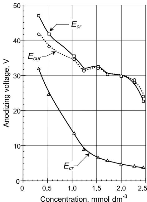
Fig. 2. Variation of anodizing voltage ( $E_{cr}$  and  $E_{cur}$  as pointed out in Fig. 1) with concentration of ammonium fluoride in aqueous  $0.4 \text{ mol dm}^{-3} \text{ H}_2\text{C}_2\text{O}_4$ . Anodizing of aluminium was performed at a constant current density of  $10 \text{ mA cm}^{-2}$ : (a) stirring off, (b) stirring in.
