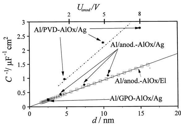
Fig. 3. Reciprocal capacity from impedance spectra as a function of the film thickness  $d$ . The corresponding anodisation potential  $U_{anod}$  is given for comparisons (formation factor  $k = 1.6 \text{ nm/V}$ ).
