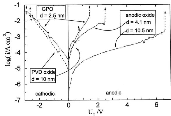
Fig. 8. Tafel plot of MIM contacts with differently prepared aluminium oxide films. The preparation method and the resulting oxide film thicknesses are given as inserts. Breakdown is indicated by an arrow symbol.
