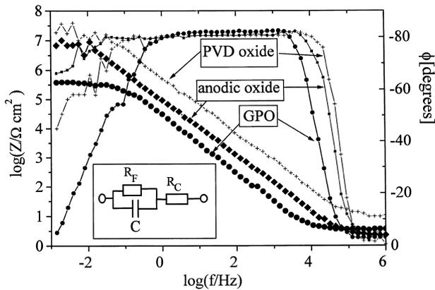
Fig. 2. Impedance spectra of Al/oxide/Ag junctions with differently prepared oxide films: gas phase oxidation (GPO), physical vapour deposition (PVD, 10 nm), and anodic oxidation (10 nm) in aqueous electrolyte.
