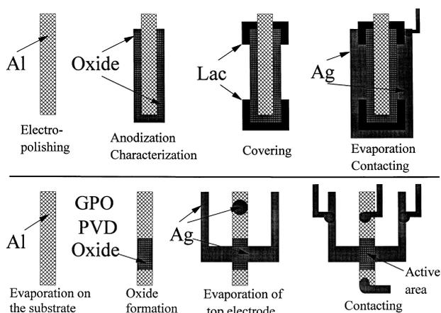
Fig. 1. Successive preparation steps of Al/oxide/Ag junctions on wires (cross-section, top) or on glass slides (top view, bottom).
