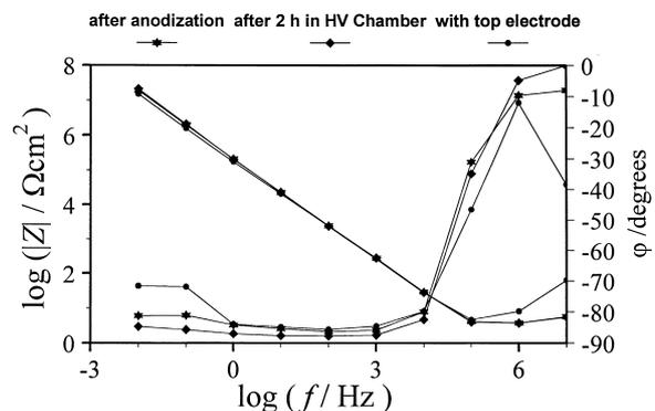
Fig. 4. Impedance spectra of wire type specimen at different stages of preparation: immediately after anodisation (Al/oxide/electrolyte), after 2 h in UHV chamber, and after evaporation of the silver top electrode.
