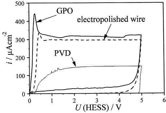
Fig. 5. Cyclic voltammograms of further oxide formation of differently prepared aluminium oxide films (GPO, PVD, electropolished Al wire) in aqueous acetate buffer. Scan rate  $dU/dt = 100 \text{ mV/s}$ .
