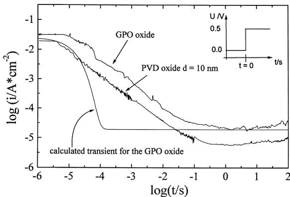
Fig. 6. Current transients of an Al/oxide/Ag junction, potential step from 0 to 0.5 V in double logarithmic presentation; comparison of GPO and PVD and a calculated transient for the GPO oxide film.
