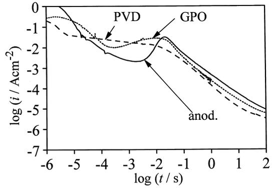
Fig. 7. Current transients of further anodic oxide formation of differently prepared oxide films for different potential steps: from 0 to 7 V for anodic oxide (10.6 nm) on an Al wire, from 0 to 0.5 V for GPO (2.6 nm) on evaporated Al, and from 0 to 5 V for PVD (10 nm) on evaporated Al.
