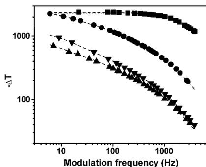
**Figure 5.** Modulation frequency dependence of the photoinduced absorption signal in Figure 3 for 40 mW laser power. (■) pristine MDMO–PPV (at 1.36 eV), (●) MDMO–PPV:9 (at 1.24 eV), (▼) MDMO–PPV:6a (at 1.24 eV), (▲) MDMO–PPV:6b (at 1.24 eV). Dashed lines show fit to monomolecular and bimolecular recombination behavior (see text).
