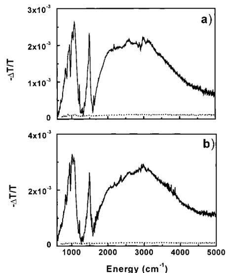
**Figure 6.** Photoinduced IRAV measurements of (a) MDMO–PPV:9 (solid line) and (b) MDMO–PPV:6b (solid line) composite films on KBr. The dotted lines in (a) and (b) show for comparison the IRAV signals for the pristine polymer film. Excitation with 488 nm at  $T = 100$ K.
