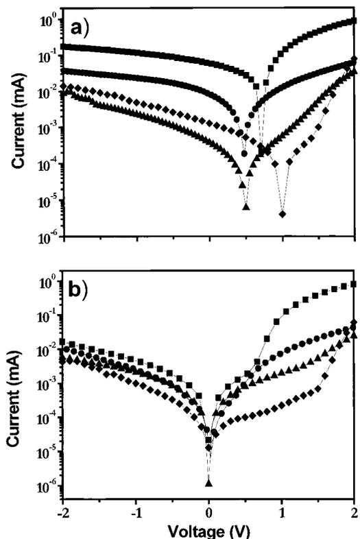
**Figure 8.** Current-voltage characteristics of different bulk heterojunction photovoltaic devices of 0.075  $\text{cm}^2$  active area. (a) Under 60  $\text{mW}/\text{cm}^2$  white light illumination and (b) in the dark. (◆) Pristine MDMO-PPV, (■) MDMO-PPV:PCBM, (●) MDMO-PPV:**9**, and (▲) MDMO-PPV:**6b** as photoactive layers.
