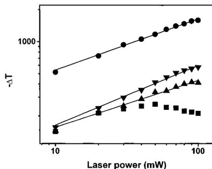
**Figure 4.** Laser power dependence of the photoinduced absorption in Figure 3 for a modulation frequency of 132 Hz: (■) pristine MDMO–PPV (at 1.36 eV), (▼) MDMO–PPV:6a (at 1.24 eV), (●) MDMO–PPV:9 (at 1.24 eV), (▲) MDMO–PPV:6b (at 1.24 eV). The solid lines show fits to a power law dependence.
