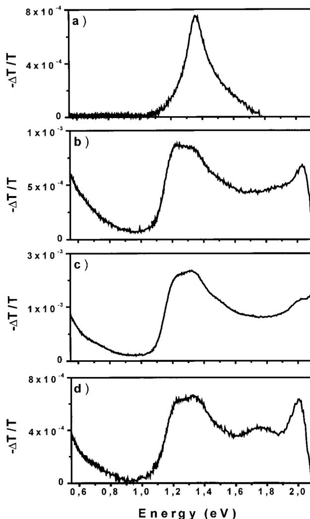
**Figure 3.** Photoinduced absorption spectra of (a) pristine MDMO-PPV film and composite (b) MDMO-PPV:**6a**, (c) MDMO-PPV:**9**, (d) MDMO-PPV:**6b** films. Excitation at 488 nm with 40 mW and 132 Hz modulation,  $T = 100$  K.
