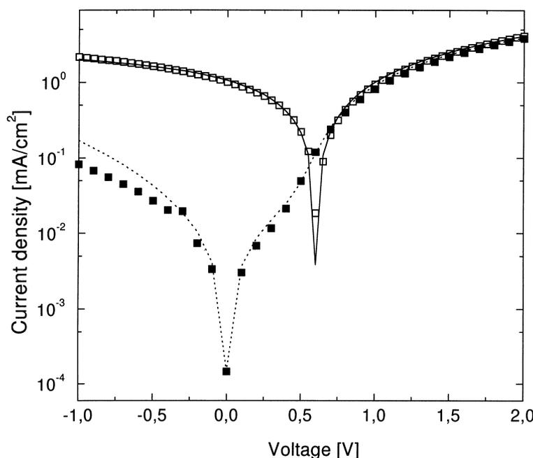
Fig. 5.  $I/V$  characteristics comparison of ITO/PEDOT/MDMO-PPV:PCBM/Al (open squares) and ITO/PEDOT/P3OT:C<sub>60</sub>/Al (solid line) under illumination with 20 mW/cm<sup>2</sup> of an argon laser (488 nm). The solid squares and the dotted line show the  $I/V$  curves of the ITO/PEDOT/MDMO-PPV:PCBM/Al and ITO/PEDOT/P3OT:C<sub>60</sub>/Al devices, respectively, in the dark.
