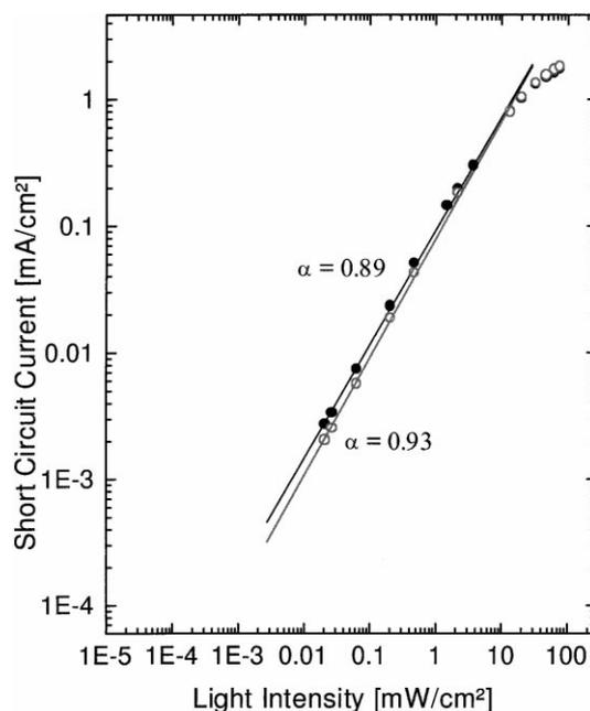
Fig. 6. Dependence of the short circuit current versus incident light intensity of an ITO/PEDOT/P3OT:C<sub>60</sub>/Al (open circles) and ITO/PEDOT/MDMO-PPV:PCBM/Al (solid circles) flexible large area plastic solar cells. Lines are fits to a power law and are discussed in the text.
