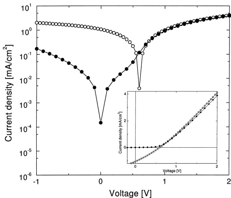
Fig. 3. Characteristics of the ITO/PEDOT/P3OT:C<sub>60</sub>/Al (solid circles: dark, open circles: illuminated with 488 nm, 20 mW/cm<sup>2</sup>) flexible large area plastic solar cell in a logarithmic scale. The inset is a linear plot of the *I/V* data for positive voltage.
