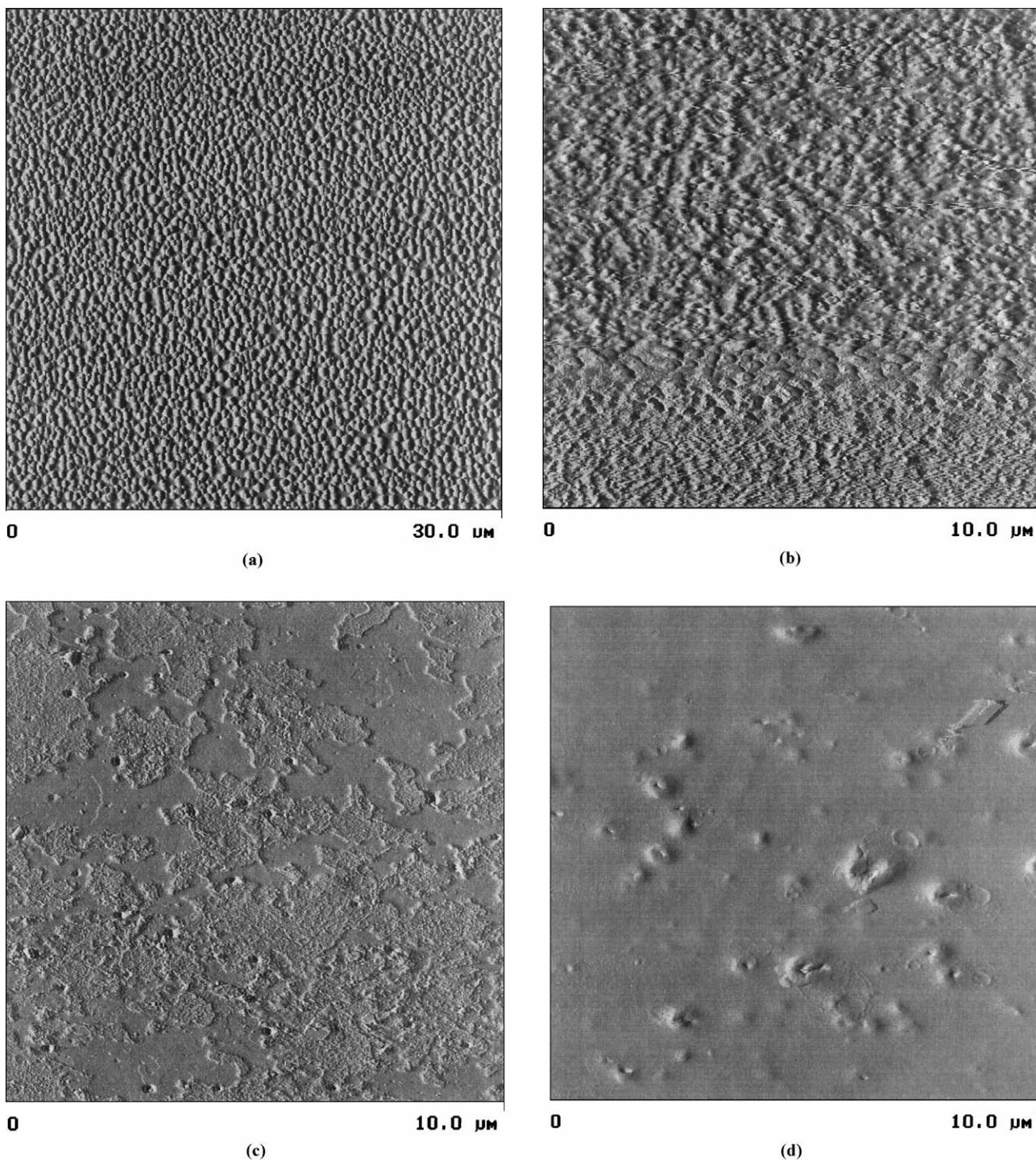
Fig. 7. AFM comparison of (a) MDMO-PPV/PCBM (1:3 weight ratio), (b) P3OT/C<sub>60</sub> (1:1 weight ratio), (c) P3OT/PCBM monoadduct (1:2 weight ratio) and (d) P3OT/PCBM multiadduct (1:2 weight ratio) composite films.
