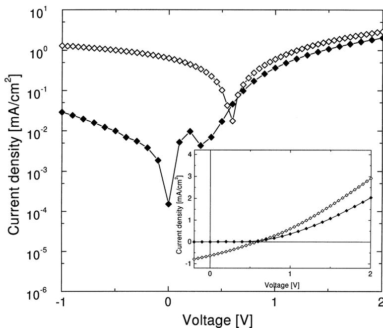
Fig. 4. ITO/PEDOT/P3OT:PCBM monoadduct/Al (solid diamonds: dark, open diamonds: illuminated with 488 nm, 20 mW/cm<sup>2</sup>) flexible large area plastic solar cell in a logarithmic scale. The inset is a linear plot of the *I/V* data for positive voltage.
