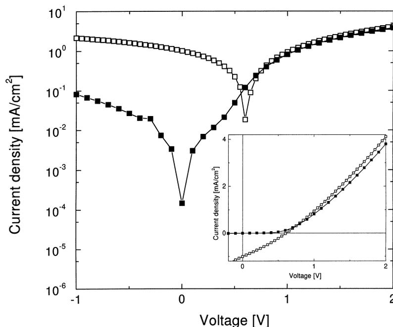
Fig. 2.  $I/V$  characteristics of ITO/PEDOT/MDMO-PPV:PCBM /Al (solid squares: dark, open squares: illuminated with 488 nm, 20 mW/cm<sup>2</sup>) flexible large area plastic solar cell in a logarithmic scale. The inset is a linear plot of the  $I/V$  data for positive voltage.
