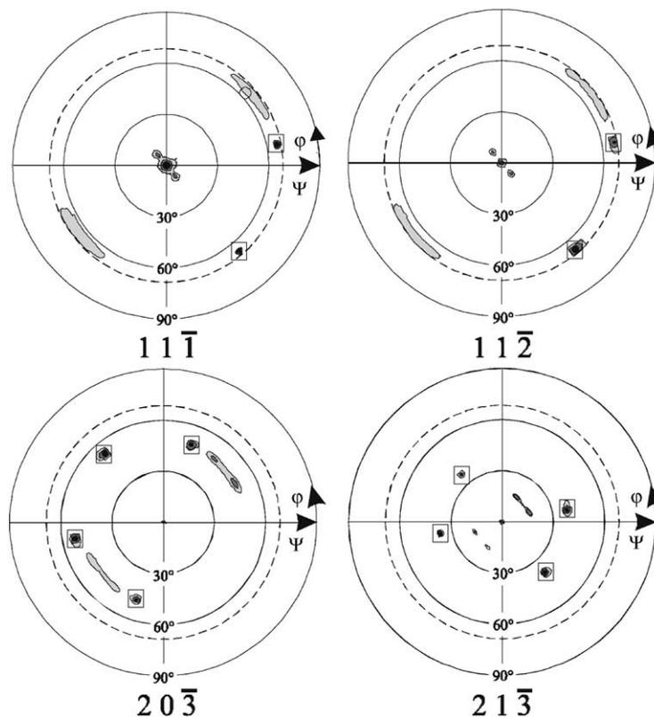
Fig. 2. XRD-PF of PSP on mica (001). The four pole figures are taken from the  $(11\bar{1})$ ,  $(11\bar{2})$ ,  $(20\bar{3})$  and  $(21\bar{3})$  reflections of PSP. The dashed line indicates the measurement limit of  $\psi = 75^\circ$ . Darker areas represent higher intensity.
