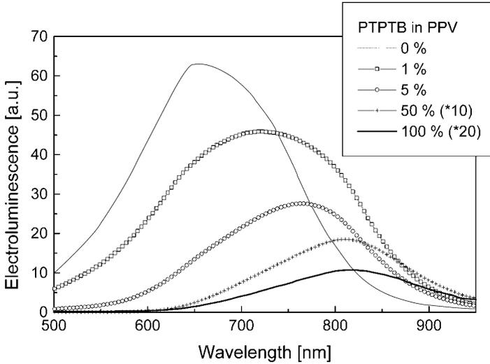
**FIGURE 4** Electroluminescence of MDMO-PPV (dotted line), PTPTB (full line) and different blends with 1% (open squares), 5% (open diamonds) and 50% (crosses) PTPTB in MDMO-PPV; electroluminescence is measured in sandwich devices with ITO/PEDOT anode and LiF/Al cathode.
