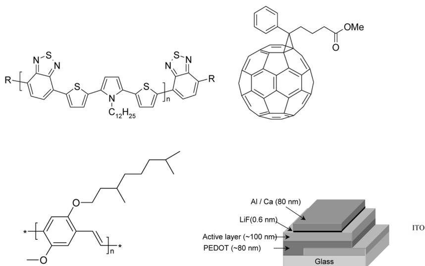
**FIGURE 1** Chemical structure of PTPTB, PCBM, MDMO-PPV and the geometric structure for the photovoltaic devices and light emitting diodes.
