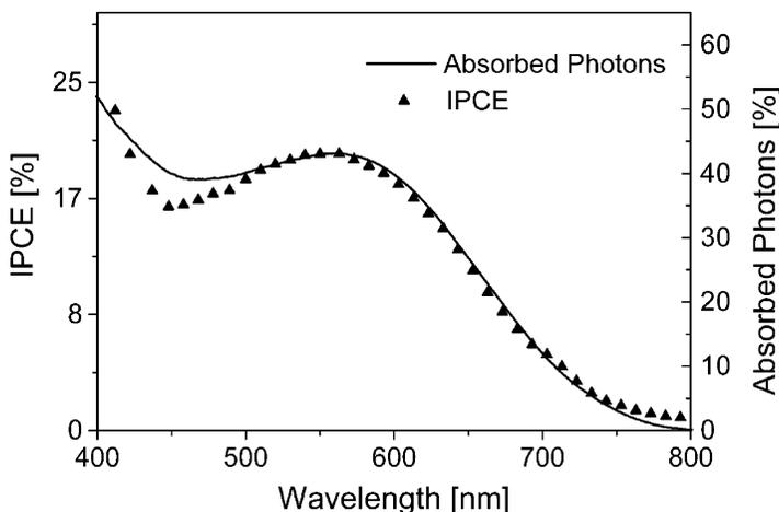
**FIGURE 6** IPCE spectrum (triangle) of a PTPTB/PCBM 1/3 device in comparison with the percentage of absorbed photons (transmission) of a reference film of comparable thickness.
