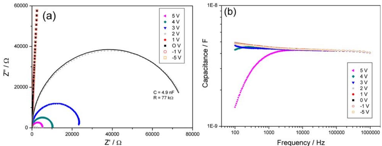
Figure 3 : (a) Cole-Cole diagram and (b) capacitance versus frequency of a MDMO-PPV diode (thickness:150 nm; surface area: 0.2 cm<sup>2</sup>) under different applied voltages.
