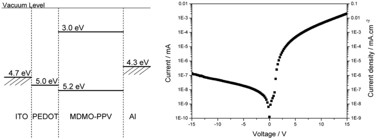
Figure 2 : (a) Energetic level diagram of the MDMO-PPV based diodes according to the MIM picture; (b) Current versus voltage graph of a MDMO-PPV diode (active surface area of 0.1 cm<sup>2</sup>).
