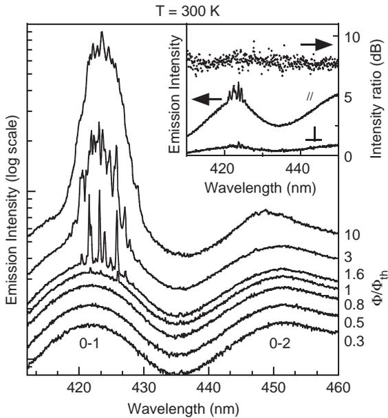
Fig. 2. Main panel: Room-temperature, time-integrated emission spectra for different values of the pump fluence  $\Phi/\Phi_{\text{th}}$ , where  $\Phi_{\text{th}} \approx 1 \mu\text{J}/\text{cm}^2$  per pulse. Inset: Emission spectra measured after polarization filtering along the direction parallel ( $//$ ) and perpendicular ( $\perp$ ) to the long molecular axis of p-6P (solid lines); Intensity ratio between the two polarization filtered spectra (dots).
