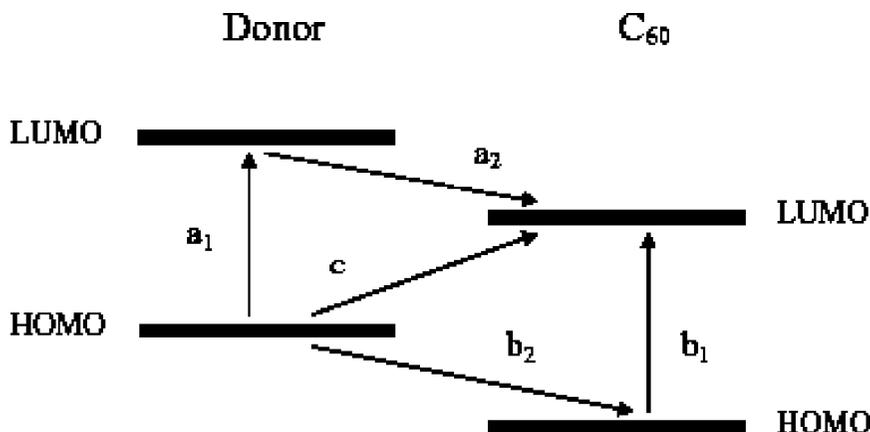
**FIGURE 10** The diagram of possible mechanisms of PIET in the C<sub>60</sub> donor/acceptor complexes: (a) excitation of the donor component; (b) excitation of C<sub>60</sub> followed by electron transfer from the donor to the excited C<sub>60</sub> molecule; (c) direct intermolecular charge transfer from the donor to the C<sub>60</sub> molecule.
