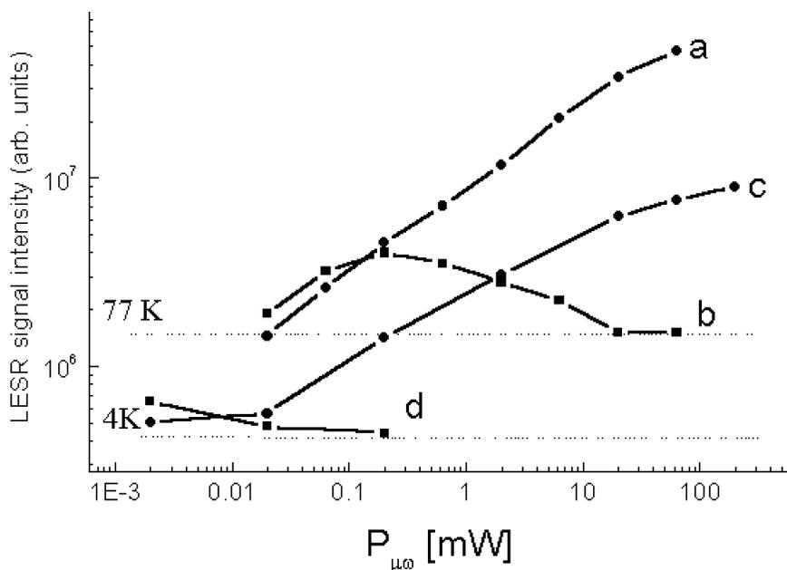
**FIGURE 4** The saturation dependencies for the LESR signals in TMPDA·C<sub>60</sub>: the high- (a) low-field (b) signals at 57 K; the high-(c) low-field (d) signals at 4 K.
