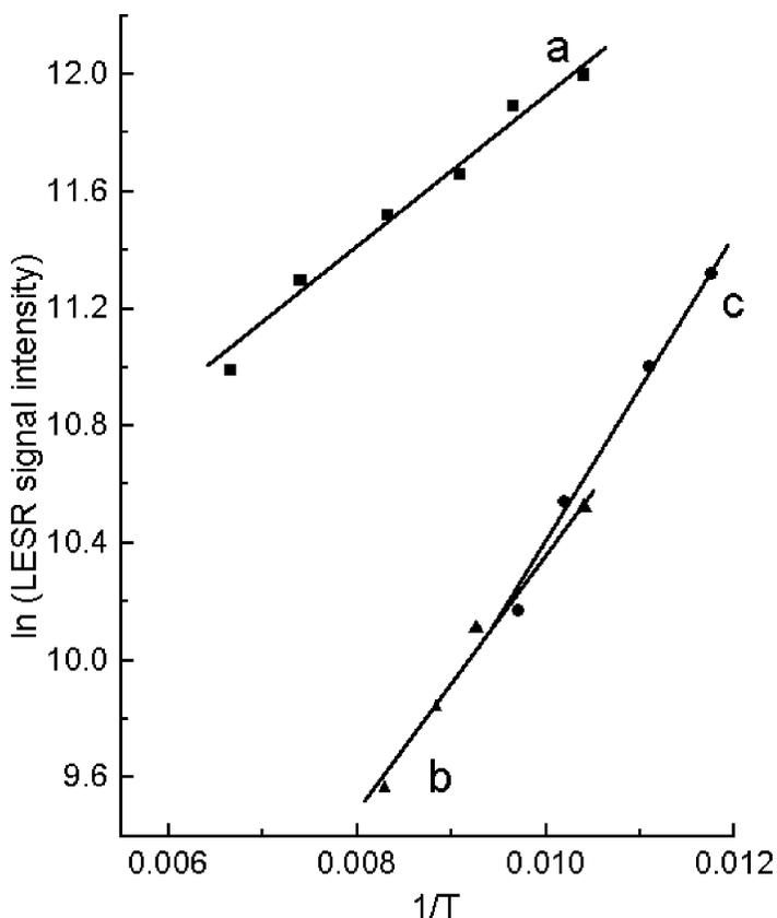
**FIGURE 8** The dependence of the hyperbolic logarithm ( $\ln$ ) of the intensity of the LESR signals vs. the inverted temperature ( $1/T$ ): (a)  $LCV \cdot C_{60} \cdot C_6H_5Cl$ ; (b)  $(BA)_2C_{60}$ ; (c)  $TMPDA \cdot C_{60}$ .
