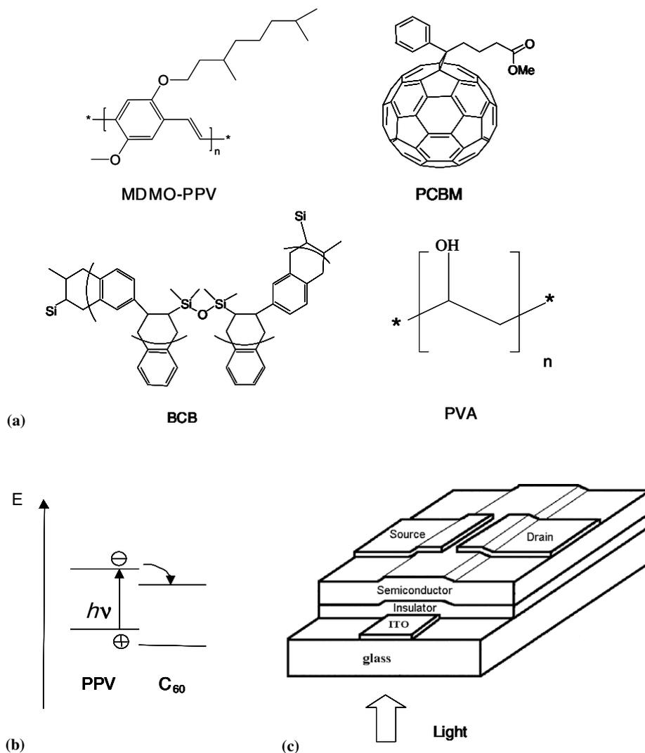
Fig. 1. (a) Molecular structure of MDMO-PPV, PCBM, BCB and PVA; (b) scheme of the photoinduced charge transfer between the PPV donor and the C<sub>60</sub> acceptor; (c) photOFET device structure.
