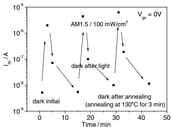
Fig. 5. Drain–source current for the MDMO-PPV:PCBM (1:4) photOFET recorded at  $V_{gs} = 0$  V in the dark, under AM1.5 ( $100 \text{ mW/cm}^2$ ) illumination, again in the dark, and after annealing, for the first three cycles.
