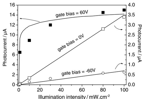
Fig. 4. Photocurrent as a function of illumination intensity in the ON-state ( $V_{gs} = 60$  V, filled square symbols), under low gate bias ( $V_{gs} = 0$  V, open square symbols) and in the OFF-state ( $V_{gs} = -60$  V, open circle symbols). Solid lines are fits using Eqs. (3) and (4).
