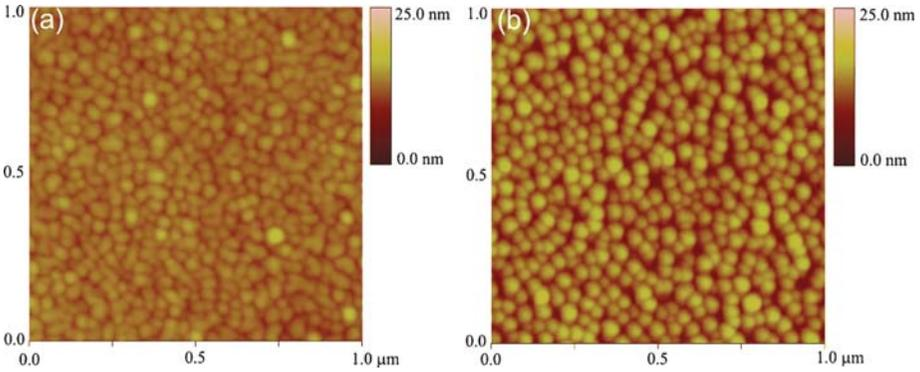
**Figure 12** AFM topography images of (a) 5-nm  $C_{60}$  film grown on BCB substrates without preheating and (b) 5-nm  $C_{60}$  film grown on BCB substrates with in-situ preheating at  $250^{\circ}C$ . Reproduced with permission from Reference 8.
