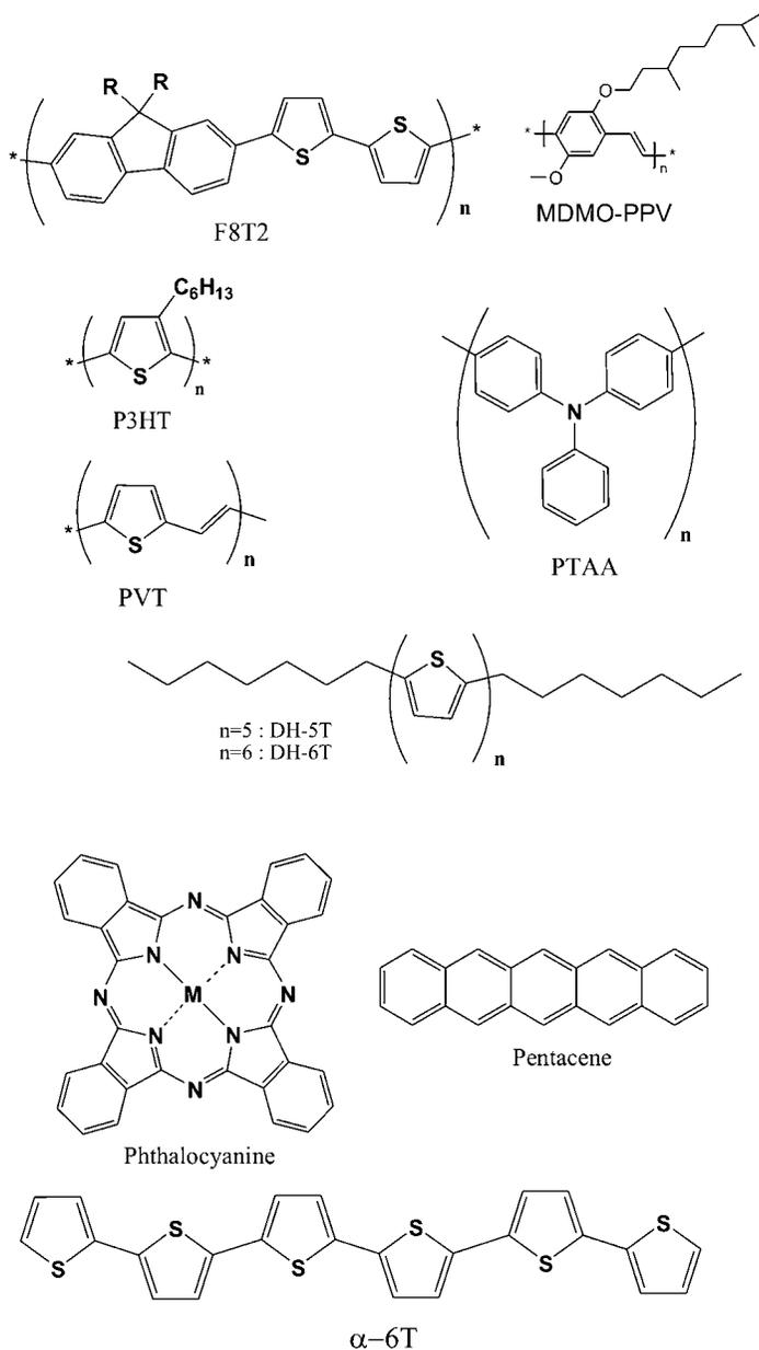
**Figure 7** Commonly used *p*-type organic semiconductors. F8T2, poly[9,9'-dioctylfluorene-co-bithiophene]; MDMO-PPV, poly[2-methoxy-5-(3,7-dimethyloctyloxy)-1,4-phenylenevinylene]; P3HT, regioregular poly[3-hexylthiophene]; PTAA, polytriarylamine; PVT, poly-[2,5-thienylene vinylene]; DH-5T,  $\alpha,\omega$ -dihexylquinquethiophene; DH-6T,  $\alpha,\omega$ -dihexylsexithiophene; phthalocyanine; pentacene;  $\alpha$ -6T,  $\alpha$ -sexithiophene.
