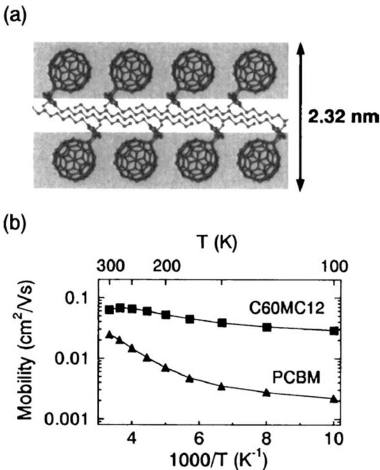
**Figure 5** (a) Illustration of schematic film structure of C60MC12 active layer. (b) Temperature dependence of the field-effect mobility extracted from the characteristics of C60MC12- and PCBM-based OFETs in the saturation regime  $V_{ds} = 50$  V. Reproduced with permission from Reference 68.
