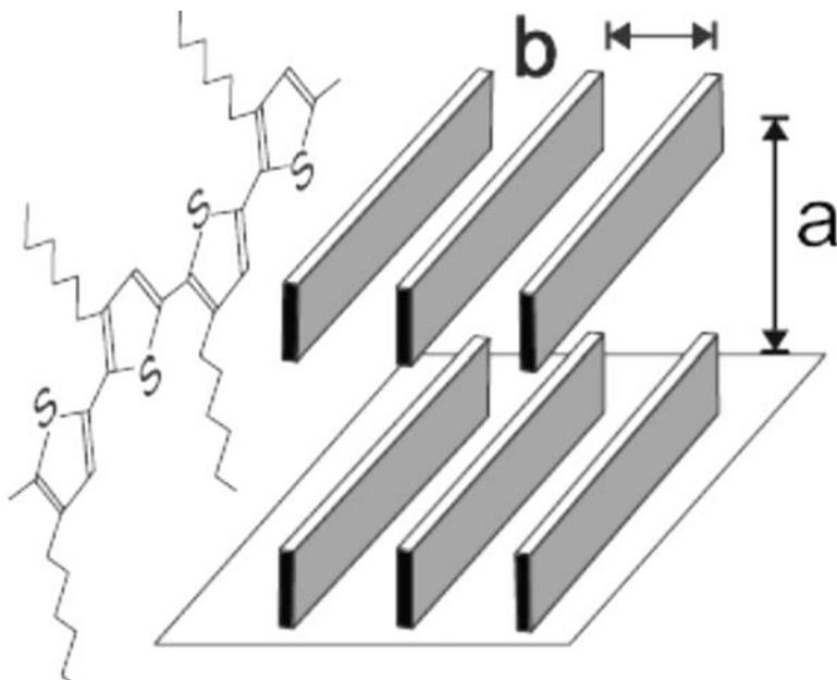
**Figure 15** Regioregular poly(3-hexyl thiophene) shows in-plane, lamellar self-organization.  $a$  and  $b$  are lattice parameters. Reproduced with permission from Reference 91.
