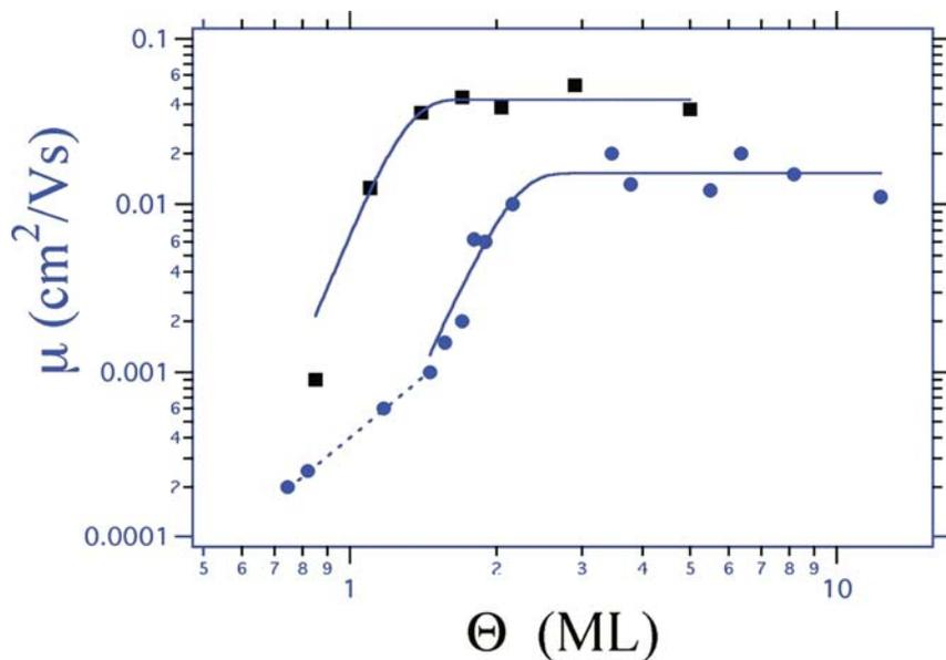
**Figure 9** Hole mobility versus coverage (number of monolayers) for low (*squares*) and high (*dots*) rates of deposition. For the high rate series, the mean value of the plateau at room temperature is  $1.5 (\pm 0.3) 10^{-2} \text{ cm}^2 \text{ Vs}^{-1}$ . A crossover from monotonic growth to the plateau occurs at  $\Theta \approx 2 \text{ ML}$ . Reproduced with permission from Reference 79.
