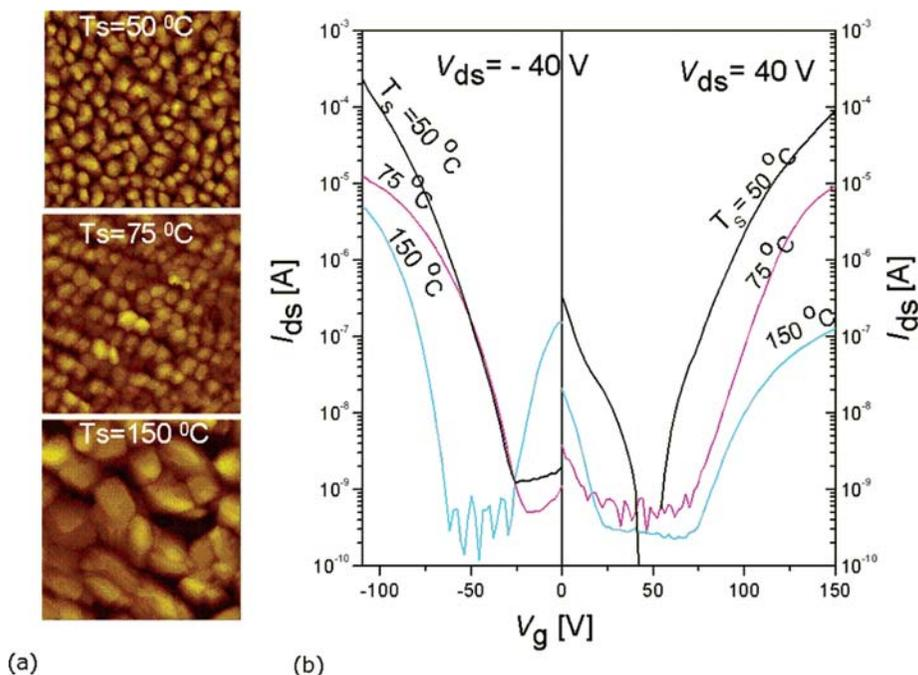
**Figure 16** (a) AFM images of pentacene film grown on polyvinyl alcohol dielectric at different elevated substrate temperatures. (b) Corresponding ambipolar transistor transfer characteristics for both electron-enhanced and hole-enhanced modes.
