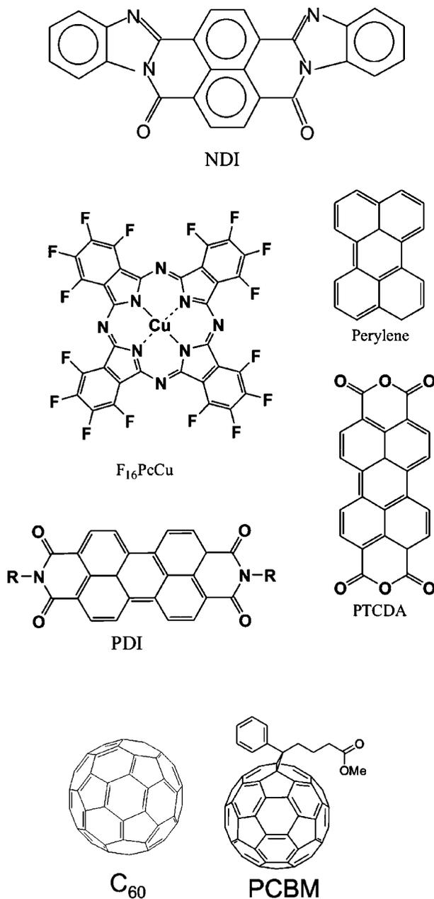
**Figure 8** Commonly used *n*-type organic semiconductors. NDI, naphthalene diimide; F<sub>16</sub>CuPc, perfluorocopperphthalocyanine; perylene; PTCDA, 3,4,9,10-perylene-tetracarboxylic dianhydride and its derivatives; PDI, *N,N'*-dimethyl 3,4,9,10-perylene tetracarboxylic diimide; C<sub>60</sub>; PCBM, methanofullerene [6,6]-phenyl C<sub>61</sub>-butyric acid methyl ester.
