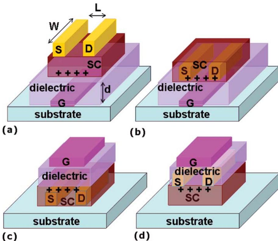
**Figure 1** Schematic of bottom-gate organic field-effect transistors (OFETs) with (a) top-contact (staggered) or (b) bottom-contact (coplanar) structures. Schematic diagram of (c) top-gate/bottom-contact OFETs using standard TFT device structures and (d) top-gate/top-contact OFETs is also shown.
