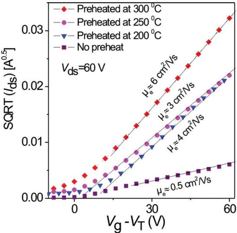
**Figure 13** Plots showing  $\sqrt{I_{ds}}$  versus  $V_g - V_T$  (symbols) for  $C_{60}$  OFETs fabricated with different growth conditions along with theoretical fit curves (without symbols) using Equation 3. The obtained electron mobilities,  $\mu_e$ , are indicated along with the respective curves. Reproduced with permission from Reference 8.
