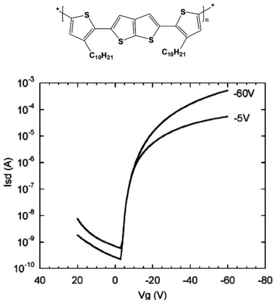
**Figure 4** (Top) Chemical structure of a polythiophene-based semiconductor incorporating thieno[2,3-b]thiophene. (Bottom) Transfer characteristics of an OFET realized using the polymer (top) as a semiconductor in air scanned from positive to negative gate voltages at drain voltages of  $-5 \text{ V}$  and  $-60 \text{ V}$ . Reproduced with permission from Reference 33.
