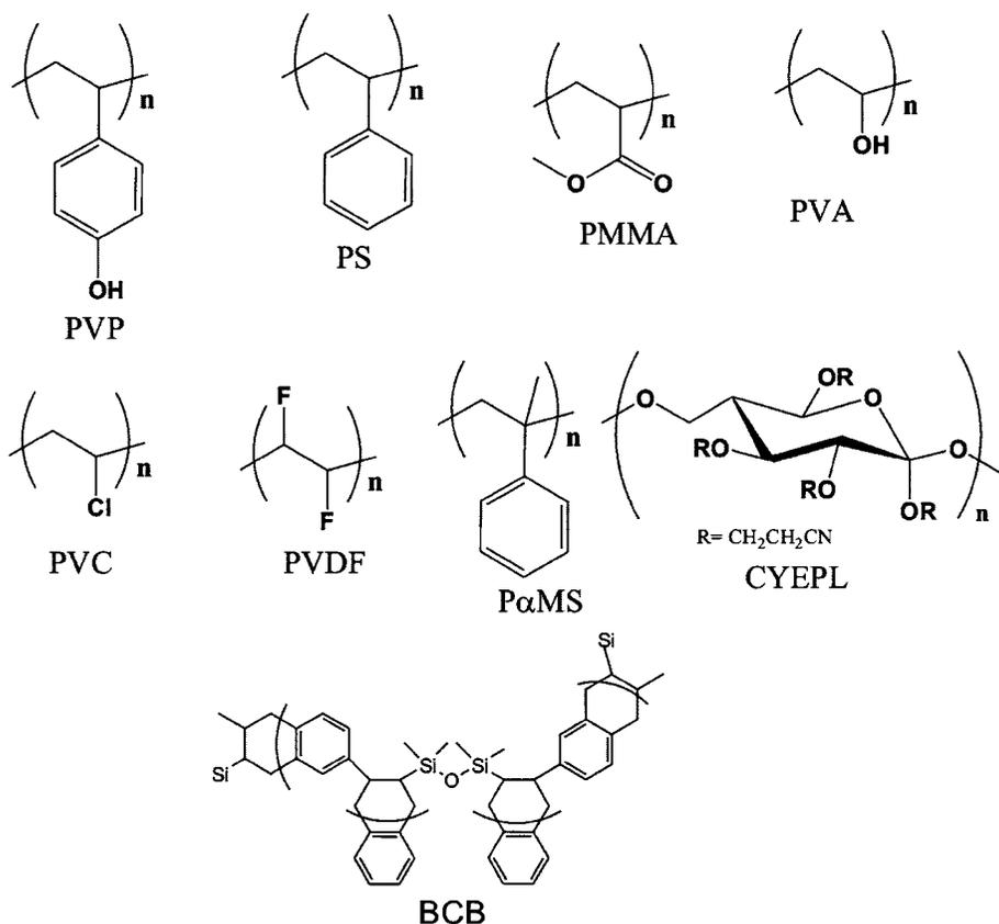
**Figure 6** Chemical structures of some commonly used organic dielectrics. PVP, poly(4-vinyl phenol); PS, polystyrene; PMMA, polymethyl-methacrylate; PVA, polyvinyl alcohol; PVC, polyvinylchloride; PVDF, polyvinylidene fluoride; P $\alpha$ MS, poly[ $\alpha$ -methylstyrene]; CYEPL, cyano-ethylpullulan; BCB, divinyltetramethyldisiloxane-bis(benzocyclobutene).
