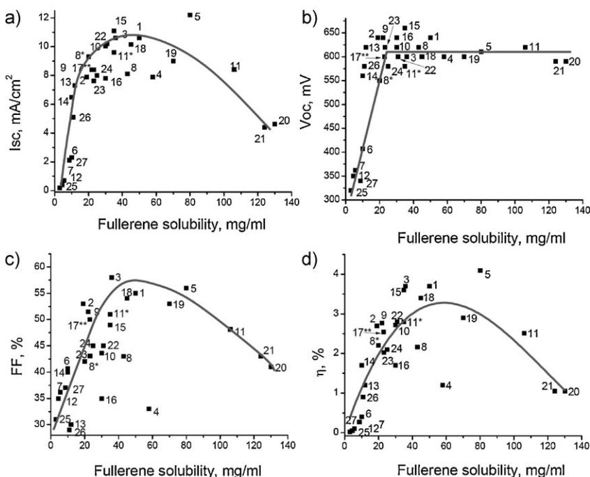
**Figure 3.** a–d) Relationship between solar cell output parameters ( $I_{SC}$ ,  $V_{OC}$ ,  $FF$ , and  $\eta$ , respectively) and solubility of the fullerene derivative used as electron acceptor material in the active layer. The lines are included as a guide for the eye.
