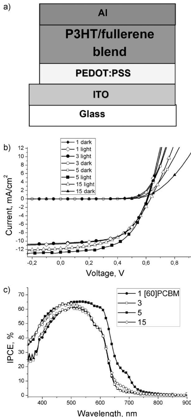
**Figure 2.** a) Schematic of the solar cell architecture; b and c) representative *I*-*V* curves and incident photon-to-current conversion efficiency (IPCE) spectra, respectively, for devices comprising different fullerene-based materials.
