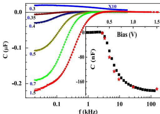
**Fig. 1.** Frequency dependent capacitance measured on an ITO-P3HT:PCBM-Al device shown for various forward bias from 0.3 to 1.5 V (as marked). Symbols: data points, solid lines: fits to the data. The 0.3 V data is multiplied by 10 for clarity. Inset:  $C(50$  Hz) vs bias voltage. Black squares – data points and red stars – fit (see text).
