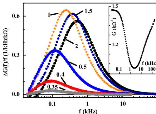
**Fig. 2.** The frequency dependence of  $\Delta G(f)/f \equiv [G(20$  Hz) –  $G(f)]/f$  for the same device as in Fig. 1, showing the typical bell shaped loss function behavior. Symbols: data points at various bias voltages (in V) as marked. Inset:  $G(f)$  vs  $f$  for  $V_{\text{bias}} = 1.5$  V.
