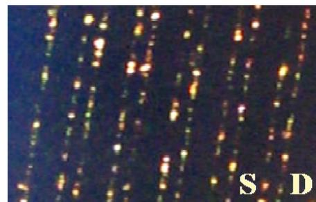
FIG. 4. (Color online) Photograph of an operating OELEFET taken through an optical microscope.
