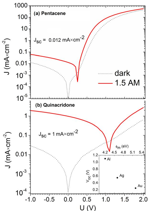
FIG. 3. Current-voltage ( $J$ - $V$ ) characteristics of ITO|PEDOT:PSS(40 nm)|semiconductor (100 nm)|Al (150 nm) diodes (a) pentacene, and (b) quinacridone in the dark and under simulated AM 1.5 illumination. The  $V_{oc}$  of quinacridone diodes with different top-contact metals is plotted versus metal work function in the inset of (b).
