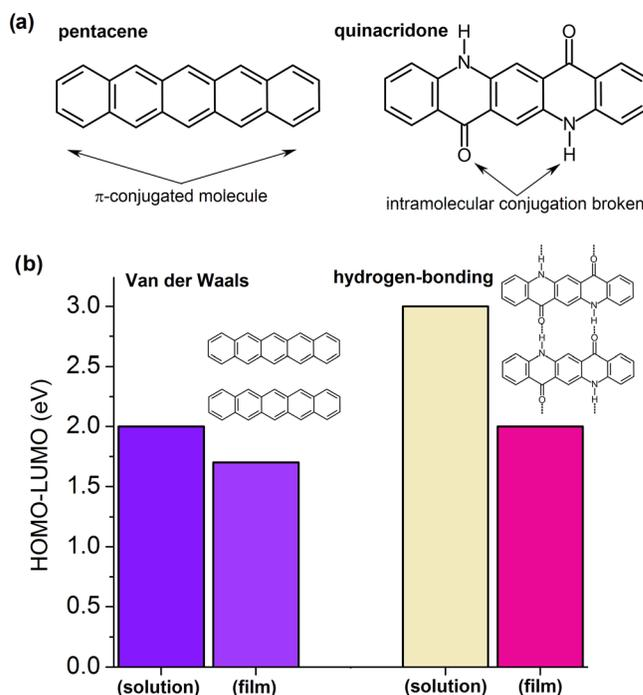
FIG. 1. (a) The molecular structures of pentacene and quinacridone. (b) The HOMO-LUMO band gap of pentacene and quinacridone, with the color of the bars representing the color of the molecules in dilute solutions and in solid state. The strong absorbance of green light resulting in red/violet colour of quinacridone occurs only in the solid state due to strong electronic coupling between neighboring molecules mediated by hydrogen bonding.
