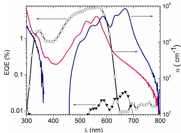
FIG. 4. External quantum efficiency (left axis) of ITO|PEDOT:PSS|semiconductor(100 nm)|Al diodes quinacridone ( $\circ$ , open circles) and pentacene ( $\blacktriangledown$ , filled triangles). Absorption coefficient (right axis) of evaporated thin films of quinacridone (pink) and pentacene (blue).
