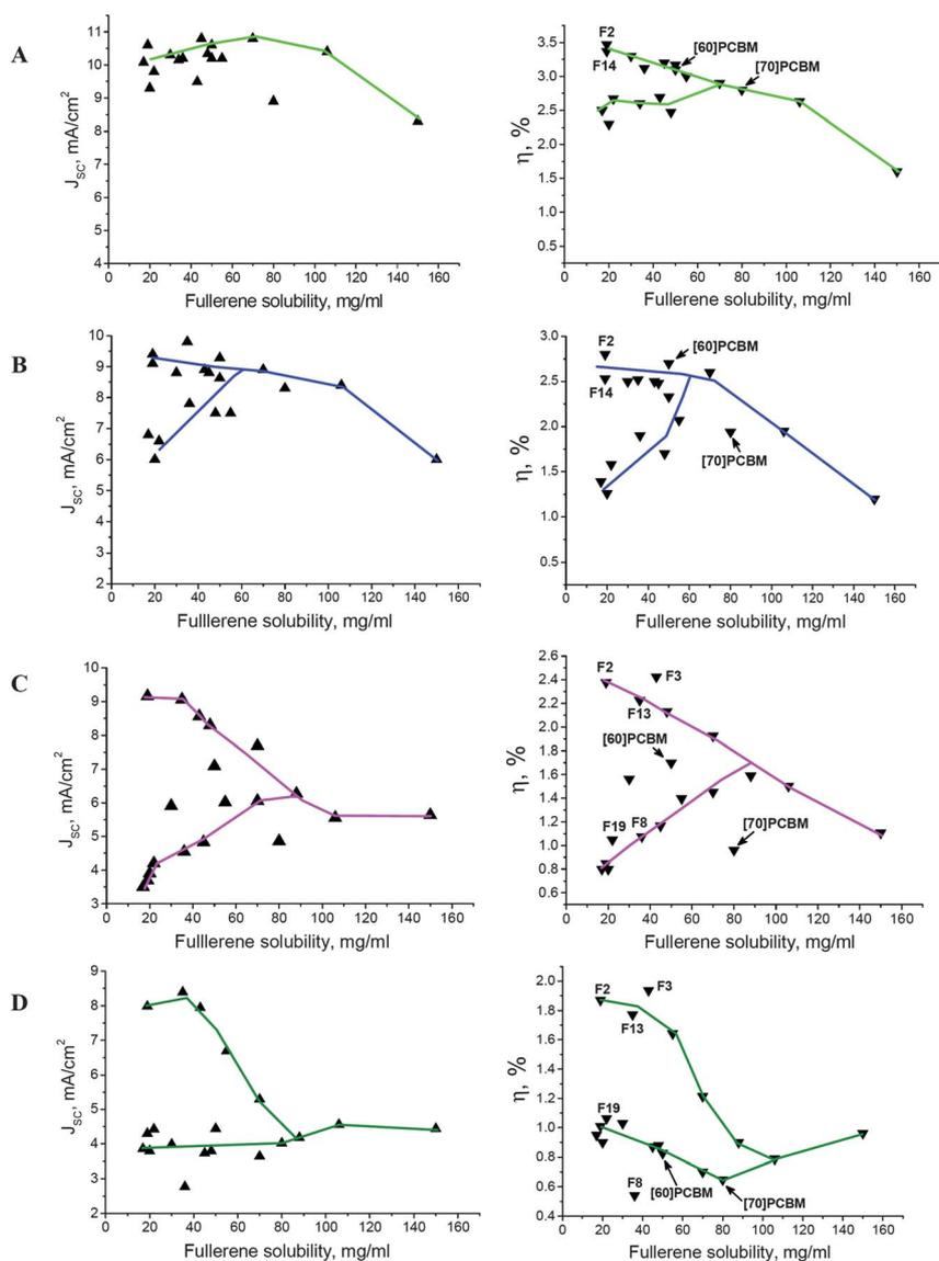
**Fig. 5** Short circuit current densities (left) and power conversion efficiencies (right) of photovoltaic devices based on P3PT (A), P3HepT (B), P3OT (C) and P3DT (D) plotted as functions of the solubility of the fullerene component. All lines are provided as guides for the eye.
