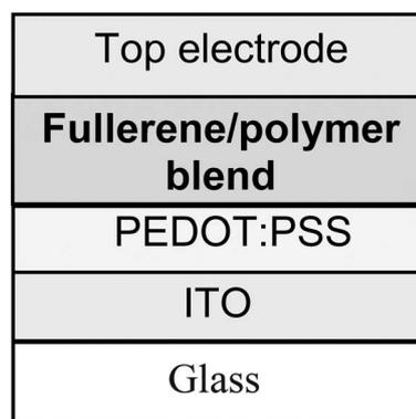
**Fig. 3** Schematic layout of the organic photovoltaic cell.
