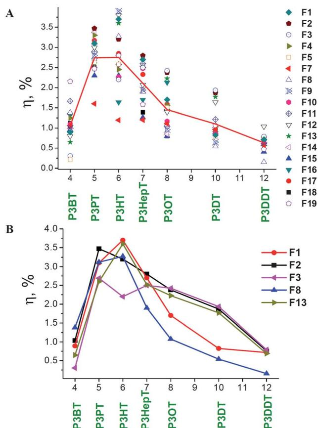
**Fig. 4** The dependence of the light power conversion efficiency on the length of the P3AT side chains in devices comprising fullerene derivatives F1–F19 (A); red line reflects the average photovoltaic performance of every P3AT with a certain alkyl chain length. Some selected dependences illustrate different behavior of various fullerene derivatives (B).
