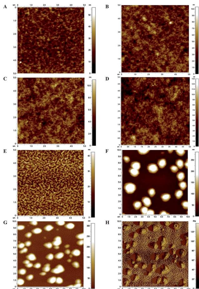
**Fig. 2** AFM height images of the composites of F8 with P3BT (A), P3PT (B), P3HT (C), P3HepT (D), P3OT (E), P3DT (F) and P3DDT (G). Phase image for the composite P3DDT (H) is provided as an additional illustration of the phase separation in the blend.
