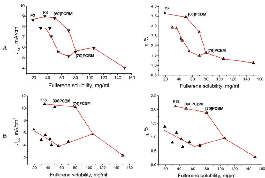
**Fig. 7** Short circuit current density (left column) and power conversion efficiency (right column) of solar cells based on the copolymers **CP-I** (raw A) or **CP-II** (raw B) and different fullerene derivatives. The red lines are provided only as guides for the eye.
