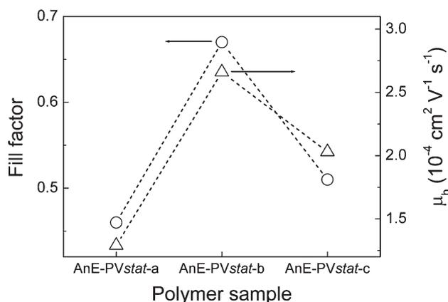
**Fig. 8** Fill factor of AnE-PVstat:PCBM solar cells (left, circles) and TOF hole mobility, at about  $1 \times 10^5 \text{ V}^{-1} \text{ cm}^{-1}$ , of pristine AnE-PVstat films (right, triangles).
