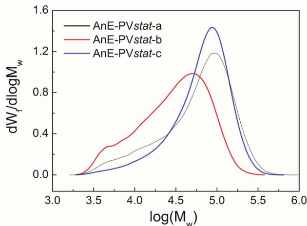
**Fig. 1** GPC curves of the three polymer samples: AnE-PVstat-a (black), AnE-PVstat-b (red) and AnE-PVstat-c (blue). THF was the mobile phase. Polystyrene standards were used for calibration.
