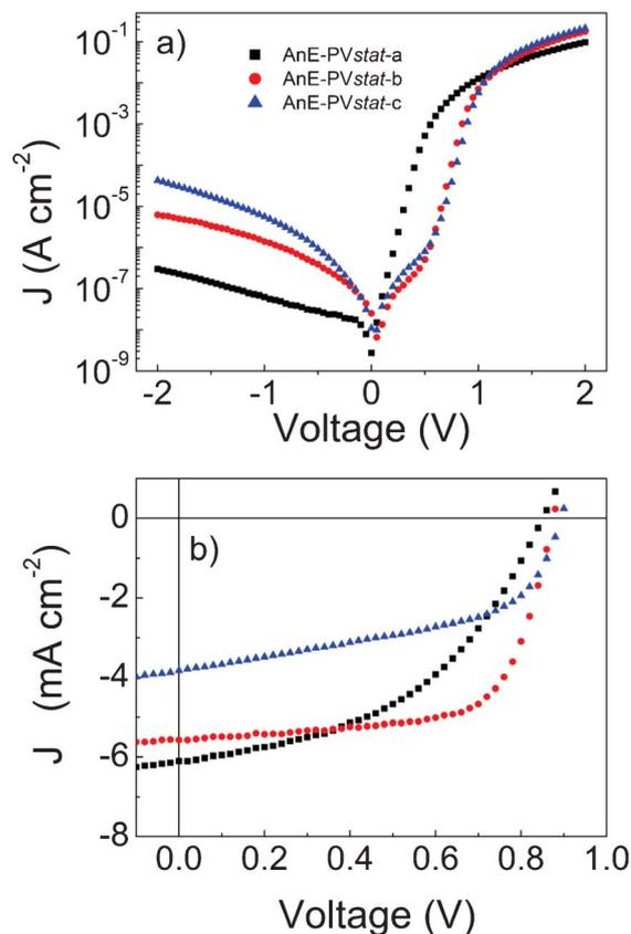
**Fig. 7** Current density–voltage characteristics in the dark (a) and under 100 mW  $\text{cm}^{-2}$  illumination (b) for solar cells made with the three electron-donors: AnE-PVstat-a (squares); AnE-PVstat-b (circles); AnE-PVstat-c (triangles).
