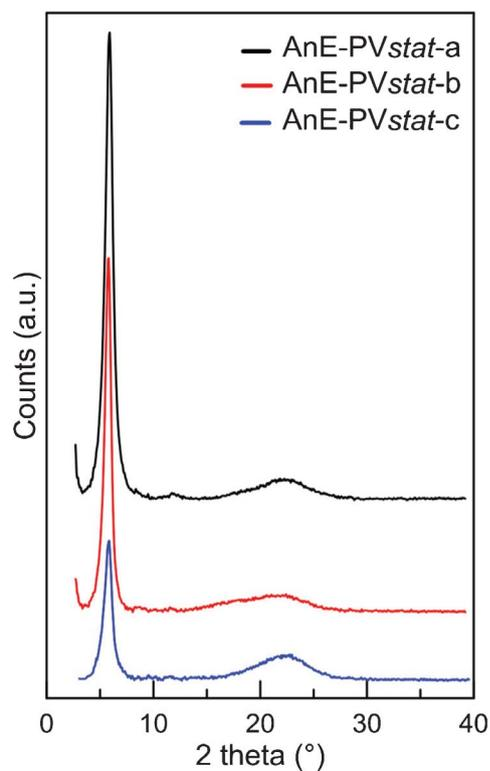
**Fig. 3** XRD patterns of films drop-cast from chlorobenzene solutions onto quartz holder.
