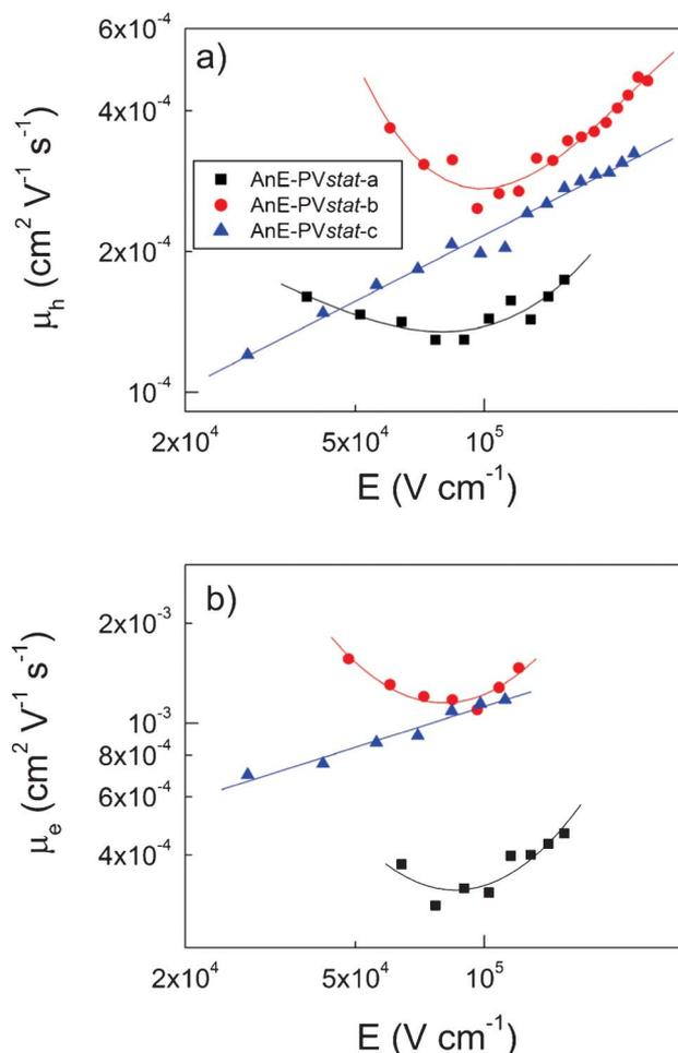
**Fig. 6** Hole (a) and electron (b) drift mobility as a function of the applied electric field: AnE-PVstat-a (squares); AnE-PVstat-b (circles); AnE-PVstat-c (triangles). Lines are shown to guide the eye.
