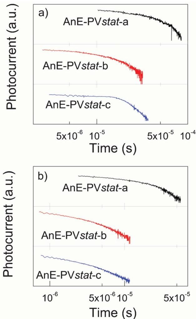
**Fig. 5** Log-log plots of photocurrent signals for holes (a) and electrons (b) for a comparable electric field of about  $1 \times 10^5 \text{ V cm}^{-1}$ .
