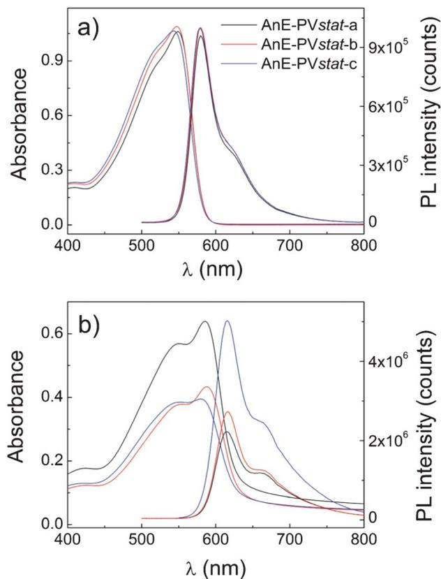
**Fig. 2** Absorption (left) and photoluminescence (right) spectra in normalized scales of a) dilute solutions and b) thin films of the same thickness (55 nm) spin-cast onto quartz substrate. The excitation wavelength was 400 nm for solutions and 450 nm for films.
