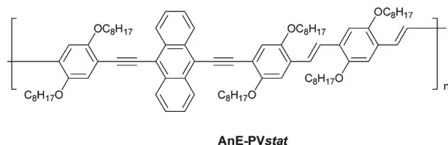
**Scheme 1** Chemical structure of AnE-PVstat (octyl =  $C_8H_{17}$  and 2-ethylhexyl =  $C_8H_{17}O$  side-chains are randomly distributed).
