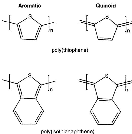
**Figure 7.2** Chemical structures of (a) PT, and (b) PITN in both aromatic and quinoid forms. The quinoid form of PITN shows an increase in aromaticity of the fused benzene ring, resulting in a much lower bandgap.
