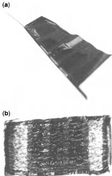
**Figure 7.4** (a) An ultrathin polymer solar cell wrapped around a human hair of radius  $\sim 35 \mu\text{m}$ . (b) An ultrathin polymer solar cell compressed on the surface of an adhesive elastomer, forming a random network of wrinkles and folds.
