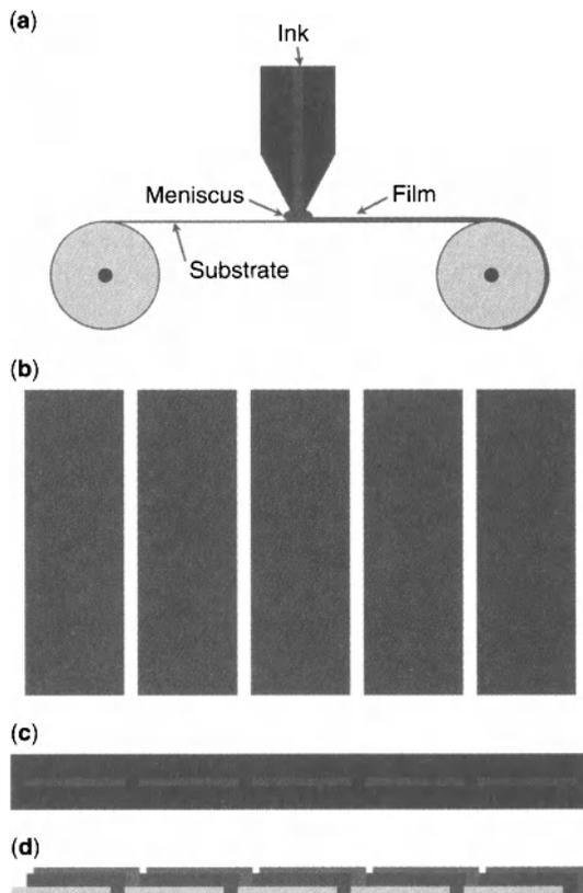
**Figure 7.5** Schematic of slot-die coating for polymer solar cell modules. (a) Cross sectional view of a roll-to-roll slot die coater. (b) Typical "parallel stripe" pattern for roll-to-roll produced polymer solar cell module. (c) One dimensional patterning in a slot-die coater, top-down view. (d) Cross sectional view of a serial-connected module, coated in the parallel stripe pattern.
