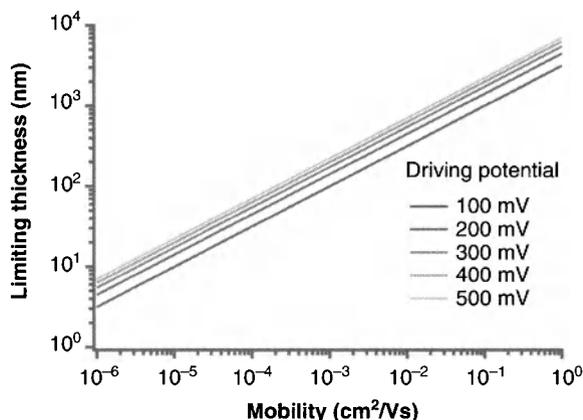
**Figure 7.3** Estimated thickness limit for a BHJ layer as a function of carrier mobility. Most semiconducting polymers limit the film thickness to roughly 100 nm.
