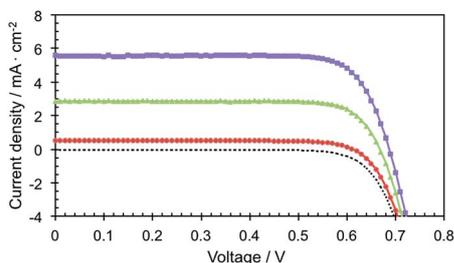
Fig. 5 Photocurrent density-voltage curves of the Zn-5-based DSSCs.
