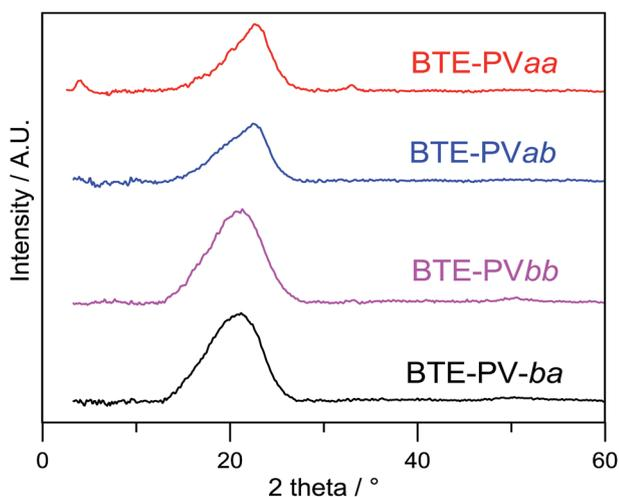
**Fig. 3** XRD patterns of polymer films drop-cast onto zero-background quartz substrate.
