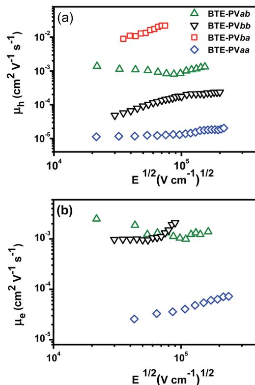
Fig. 2 Hole mobility (a) and electron mobility (b) as a function of the square root of the electric field for: **BTE-PVaa** (blue diamonds); **BTE-PVab** (green triangles); **BTE-PVba** (red squares); **BTE-PVbb** (inverted triangles).
