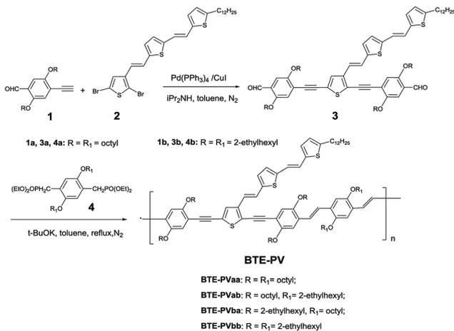
Scheme 1 Synthesis of monomers (3a, 3b) and of conjugated polymers BTE-PVs.
